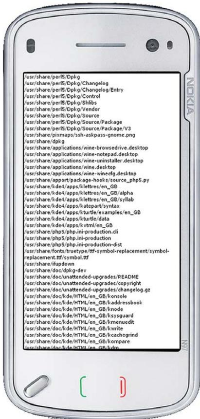
Figure 2. Output of a find Command on the Nokia N97
