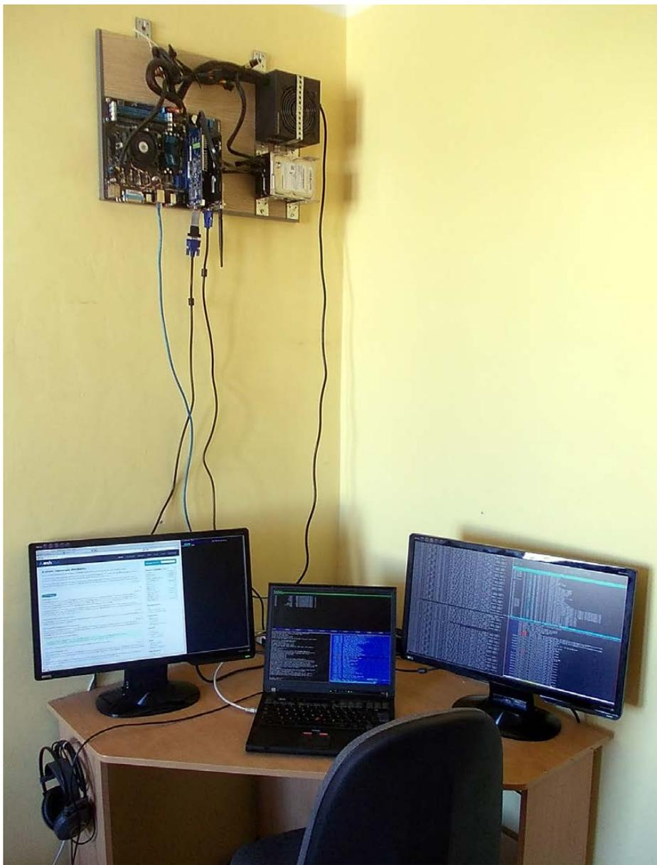
Figure 1. VMS (Virtual Machine Server): a wall-mounted, dual-head PC and a laptop connected with Synergy.
