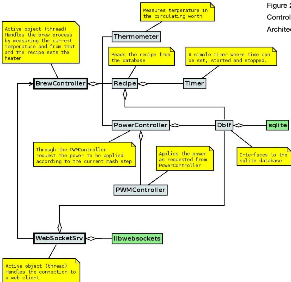
Figure 2. Brew Controller Software Architecture
