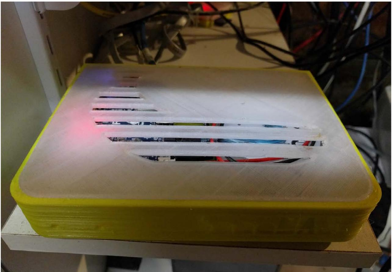
Figure 1. The Banana Pi NAS Case with Lid
