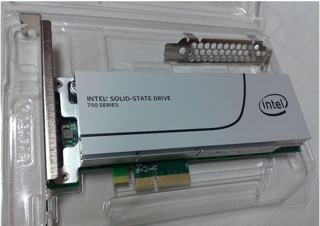
Figure 7. A PCIe NVMe SSD (by Dsimic - Own work, CC BY-SA 4.0, <https://commons.wikimedia.org/w/index.php?curid=41576100>)
