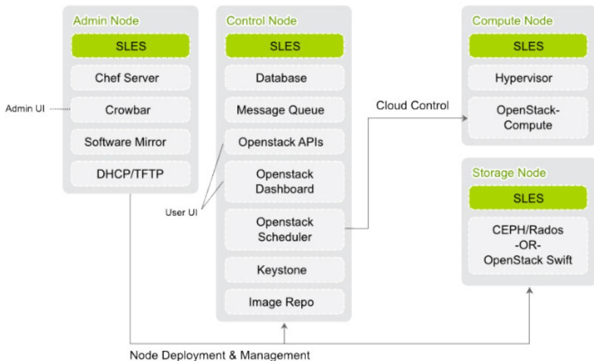
**FIGURE 2.** A General Overview of SUSE OpenStack Cloud Infrastructure (Image from SUSE OpenStack Cloud Documentation)
