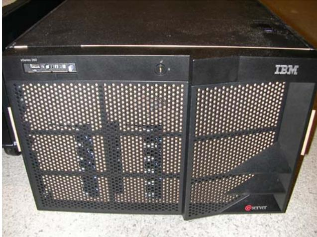
2.10 Place PolyBag (37L0557) over top of unit. Once bag is on, tuck one end of the bag under the unit between the front and rear wheels and pull through to the opposite side, eliminating any slack in the bag. Place IBM logo tape on end of bag that was pulled through under the unit and seal shut.
