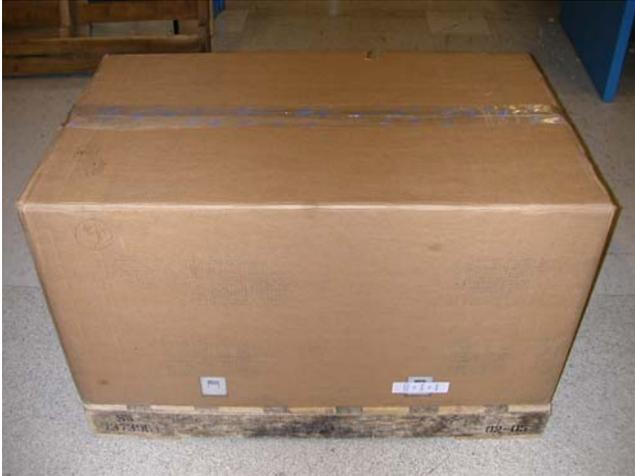
2.23 Place Intel label (if called out in DFC) on the top of the carton between label location marks.
