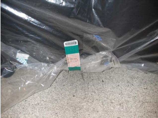
2.12 Place unit in bottom cushions. Make sure system is positioned all the way down and not sitting on the cushion ledge.
