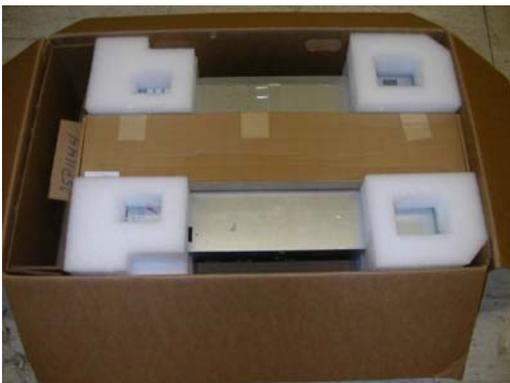
2.19 Place appropriate shipgroup content inside shipgroup divider and fold shipgroup divider flap down. Place power cords on top of divider flap.
