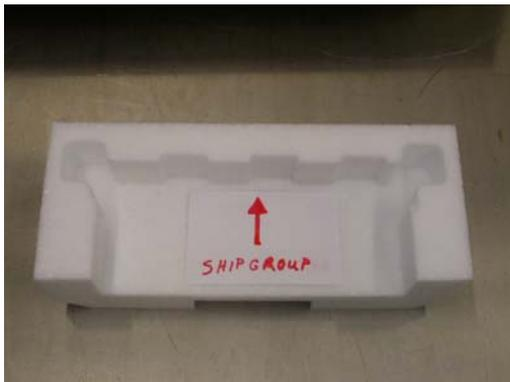
2.8 Place rear load spreader (25P1145) on rear of system as shown. (Scan Barcode if prompted by DFC).
