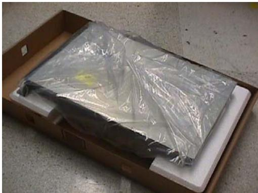
2.10 Seal edges of Bag closed with Tamper Label (06P6550).
