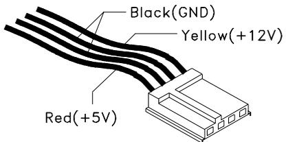
Figure 5-5 3.5-In. Diskette Drive Power Cable Connector
