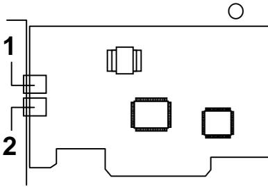
Figure 5-6 Factory-Installed Modem Card Layout
