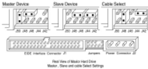
Figure 5-7 3.5-In. Hard Disk (Maxtor) Jumper Settings Locations
