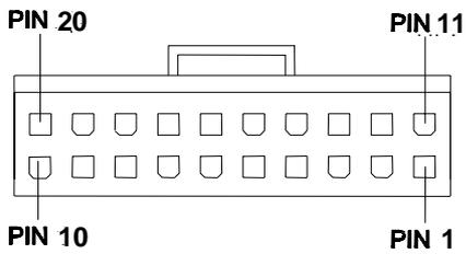
Figure 5-3 System Board Power Supply Connectors
