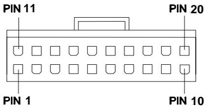
Figure 2-1 Power Supply Connectors (Bottom View)
