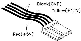
Figure 2-3 3.5-In. Diskette Drive End of Power Cable
