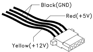
Figure 5-4 Hard Drive or CD-ROM Power Cable Connector
