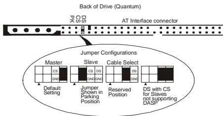
Figure 5-8 3.5-in Hard Disk (Quantum) Jumper Settings Locations
