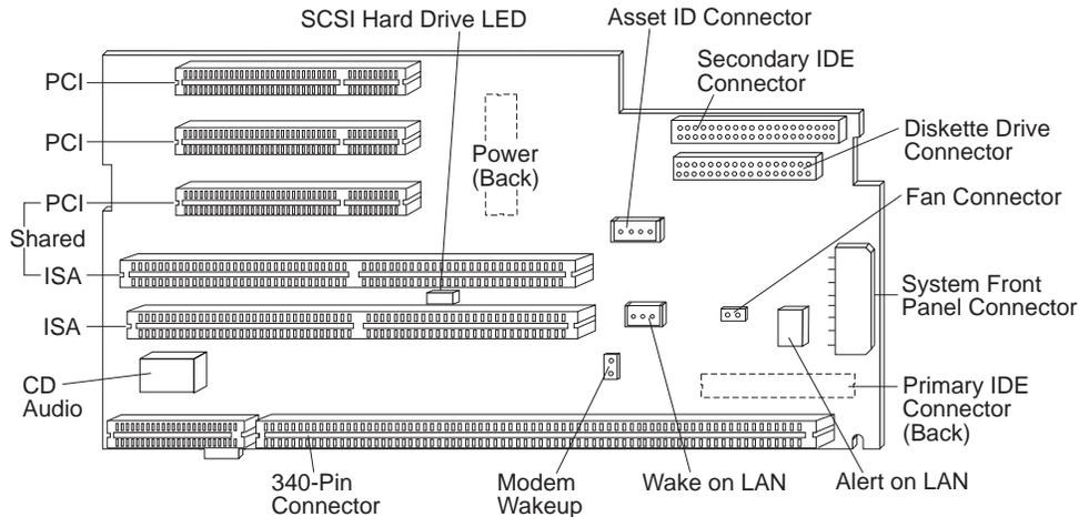
Each PCI-expansion connector is capable of driving one, low-power Schottky load. Each ISA-expansion connector is capable of driving two, low-power Schottky loads. The ISA bus is permanently set to the PCI bus speed divided by four.
