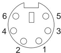
Figure 42. Mouse and Keyboard Port Connector Pin Assignments
