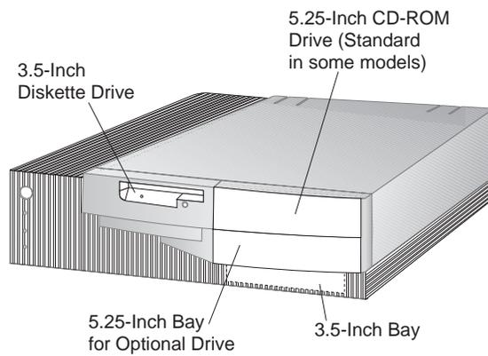
**Tower Model Drive Bays:** Your computer has six drive bays. Unoccupied drive bays can be used for installing additional devices such as hard disk and CD-ROM drives. The following illustration shows the drive bays in your computer.
