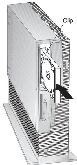
1. Close the tray by pressing the Eject/Load button, or by gently pushing the tray forward. When the tray is closed, the indicator light on the front of the drive will activate to indicate that the drive is in use.
