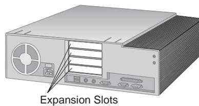
**Tower Model Expansion Slots:** Your computer has six expansion slots. One or more of these slots might be occupied, depending on the model of your PC. Unoccupied slots can be used for installing adapters. The following illustration shows the locations of the expansion slots.
