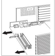
$\bf 3$  Remove the bottom expansion slot screw and cover.
