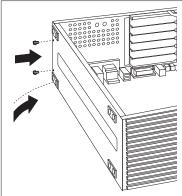
${f 4}$  Align the holes and insert the two bottom screws.
