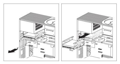
**2** Disconnect the cable from the hard disk drive in bay 6. If there is a drive in bay 5, disconnect its cable.
