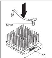
${f 9}$  Press down on the loop to rehook the clip to the tabs on the connector.
