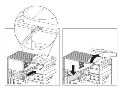
**3** Remove the top-handle screw and the screw from the drive support bracket that hold the drive cage for bays 1 through 4 in place. Then, pull the drive cage towards the power supply until it stops, and then lift it out of the computer.
