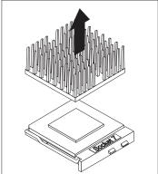
**4** Release the lever on the side of the microprocessor connector and lift it all the way up. This releases the microprocessor. Lift the microprocessor out of the socket.
