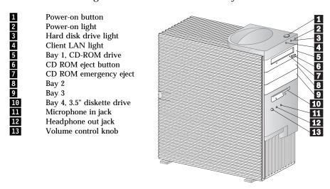
Your computer comes with a diskette drive installed in bay 4 and a hard disk drive installed in bay 6. If your computer comes with a CD-ROM drive, it is installed in bay 1; if your computer comes with a SCSI adapter, it is installed in an expansion slot.
