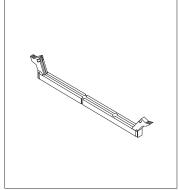
**3** Touch the static-protective package containing the memory module to any *unpainted* metal surface in the computer, and then remove the module.
