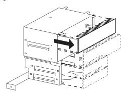
Note: If you remove a drive which has removable media from a bay and you do not intend to install a new drive immediately, replace the bay panel and the metal shield.
