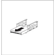
If you are installing a drive, slide the drive into the bay and secure it with the screws.
