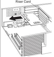
${f 2}$  Remove the adapter and insert it into a static-protective package.
