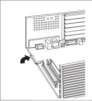
Because you cannot see the connection with the full-sized adapter in place, it is important to engage the system board latch in the support to make sure it is fully seated.
