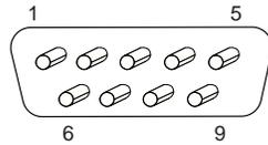
Figure 13. Serial Port Connector
