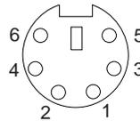
Figure 14. Keyboard and Mouse Port Connector
