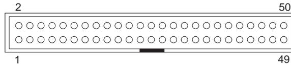
Figure 8. SCSI 50-pin Connector
