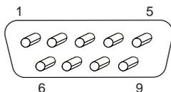
Figure 11. Serial Port Connector
