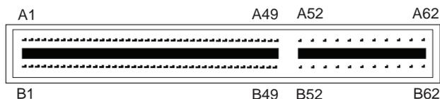
Figure 5. PCI Bus Connector
