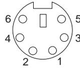
Figure 13. Keyboard and Mouse Port Connector
