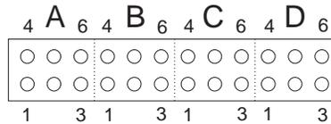
Figure 3. Pin Layout for the System Board Jumper Blocks
