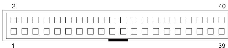
*Figure 21 (Page 1 of 2). IDE connector pin assignments*
