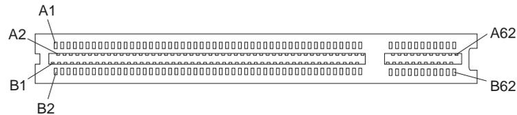
*Figure 19 (Page 1 of 3). PCI connector pin assignments*
