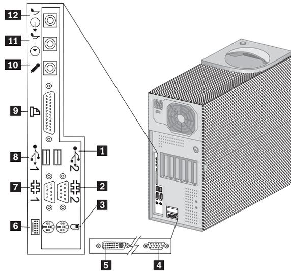
The following illustration shows the connector panel for the desktop model:
