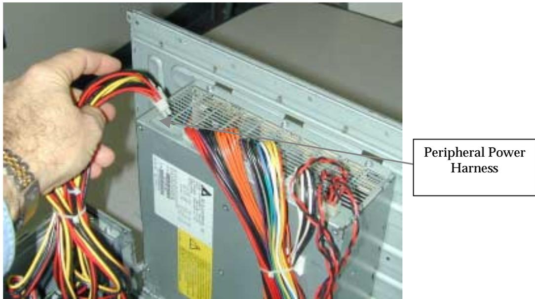
*Figure 3 Peripheral power harness*
