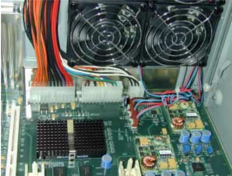
*Figure 10 Main-power connection to baseboard (rear)*
