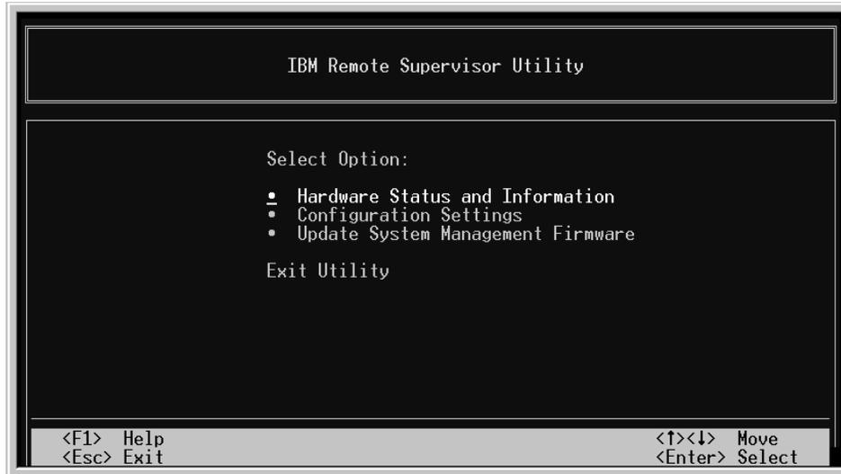
4. Use the Up Arrow and Down Arrow keys (↑ and ↓) to select **Update System Management Firmware**; then, press Enter. A warning window opens.
