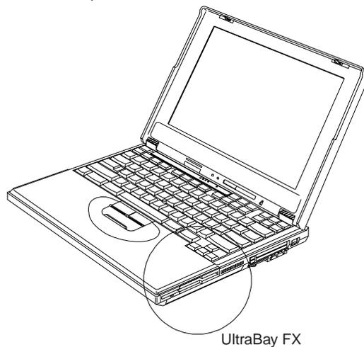
The UltraBay FX allows you to use a variety of devices with your computer. With the UltraBay FX, you can swap in new devices (such as upgraded drives or a second battery) to get the most flexibility from your computer. You can install the following drives or devices in the UltraBay FX:
