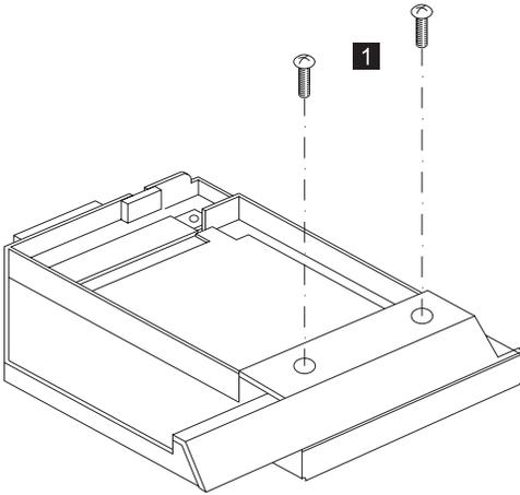
2. Slide the hard disk drive out and up to remove.
