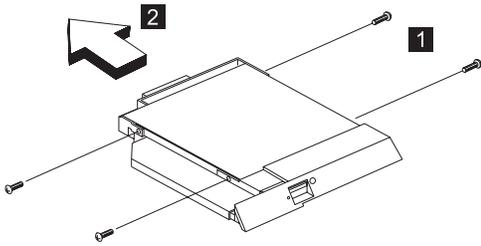
2. Carefully slide out the CD-ROM ASM to remove.
