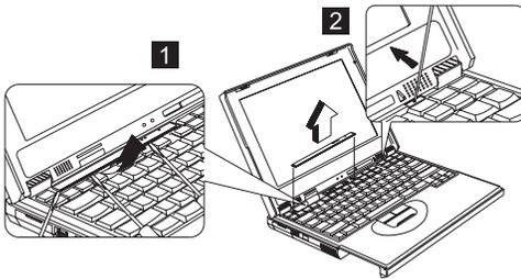
2. Remove the two screws securing the keyboard.
