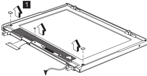
Remove the three screws securing the LCD bezel.
