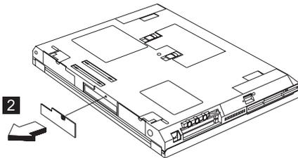
3. Carefully slide out the hard disk drive module to remove.
