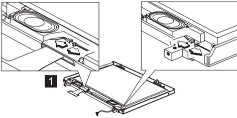
2. Remove the five screws securing the speaker.
