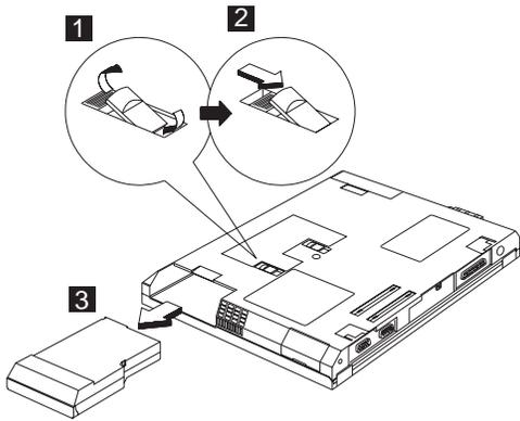
Reverse the steps described above when installing a new battery pack.
