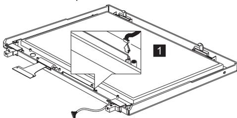
2. Carefully remove the VR board from the display panel.
