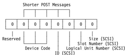
Each SCSI device is assigned a unique SCSI ID. Duplicate SCSI ID settings can generate a false error message. Use the SCSI ID to determine whether an error message is coming from an internal or an external device.
