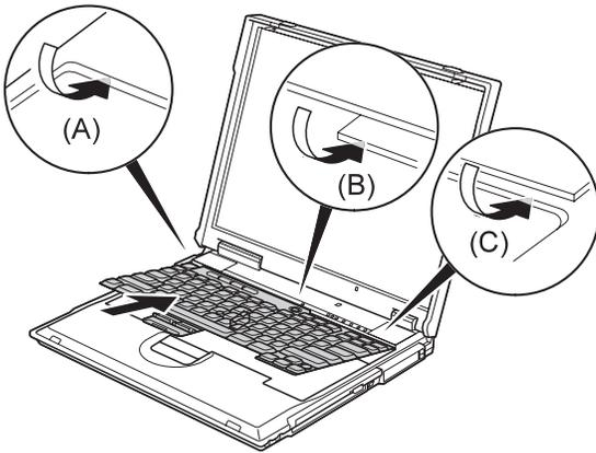
2. Push the **Y** key **1** to connect the keyboard to the connector on the underside of the key; then push the frame of the keyboard **2** to latch the latches.
