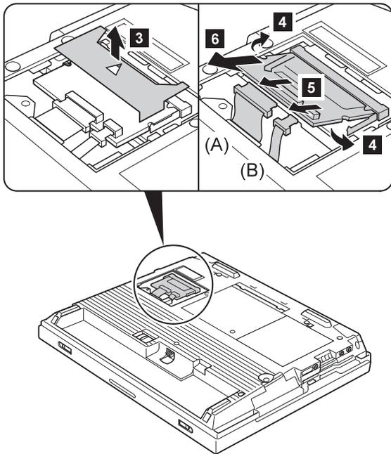
**Note:** The illustration shows the combo card. Connector **(A)** is for the LAN feature and **(B)** is for the modem. This slot also supports a Mini PCI modem card or Mini PCI network card. Step **5** depends on the card type. Disconnect either **(A)**, **(B)**, or both.
