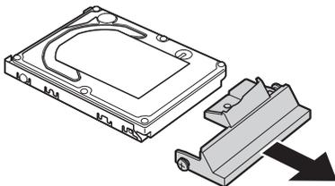
**When installing:** Make sure that the HDD connector is firmly connected.
