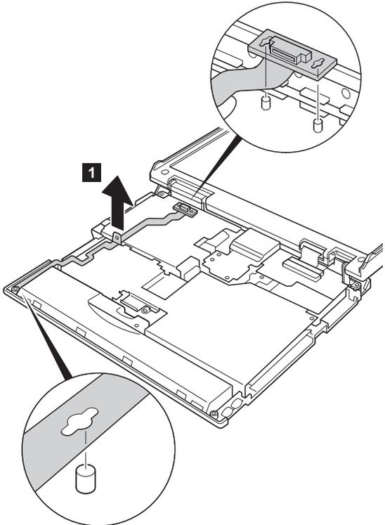
**When installing:** Make sure that you fasten the connector firmly.
