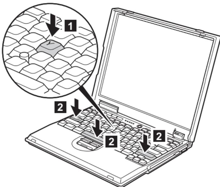
3. After the fastening of two screws of bottom side, push the **Y** key again to connect the keyboard firmly to the connector on the underside of the key.
