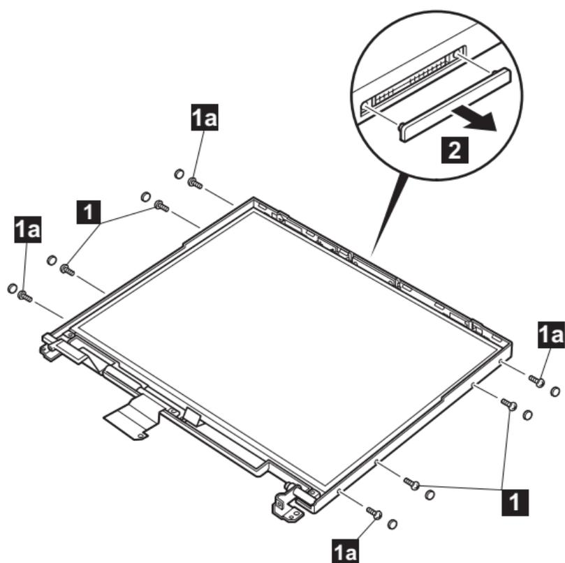
**1** for 13.3-in.LCD, LG (05K9636) and 14.1-in.LCD, Hitachi (05K9568)
