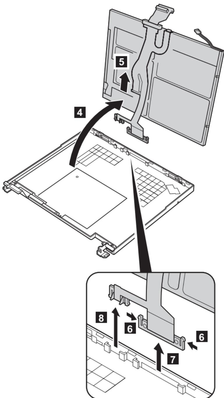
**Cable routing:** When installing the LCD, see the following figure for the routing of the connector cable.
