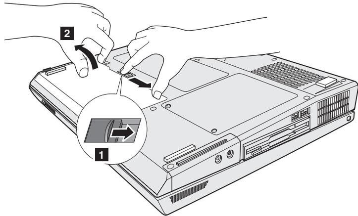
4. Align the side of a fully charged spare battery with the side of the battery space in the computer **1**; then gently push the battery into the space **2**.
