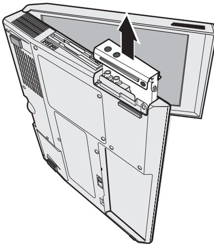
6. Do not remove the screws from the sides of the cover; instead, detach the cover from the hard disk drive by pulling in the direction of the arrows, first **1** and then **2**.
