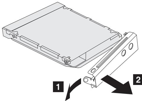
7. Attach the cover to a new hard disk drive.
