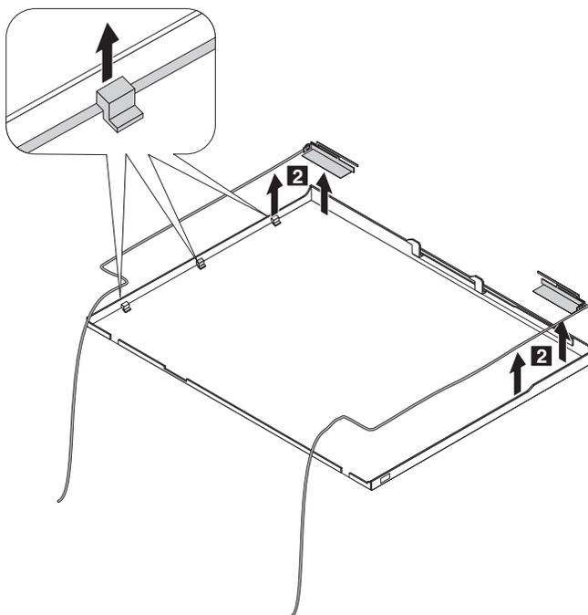
**Note:** For models without wireless WAN, the only antenna present on the right-side is the aux wireless LAN antenna.
