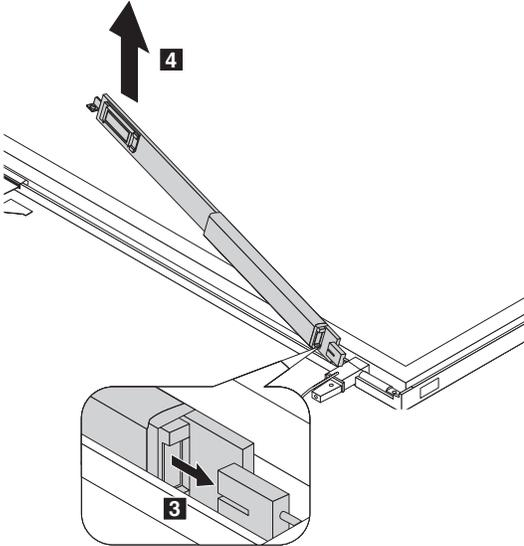
**When installing:** Make sure that both connectors are attached firmly.
