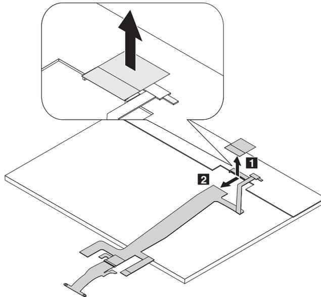
**When installing:** Make sure that the cable is positioned correctly, the connector is attached firmly, and the tape is reattached.
