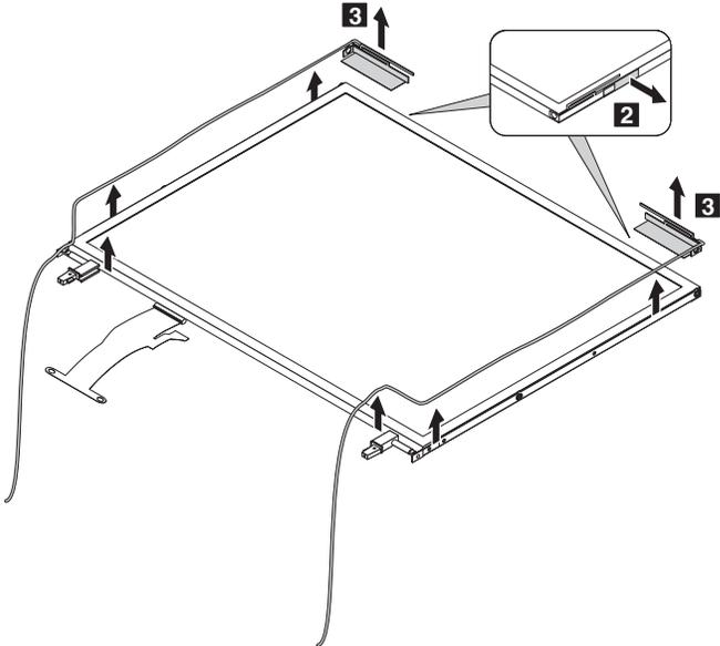
**When installing:** Route the cable properly along the side and into the hinge.
