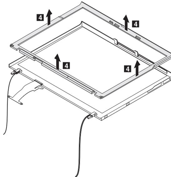
**When installing:** The replacement bezel should have adhesive pre-applied; therefore, remove the covering from the bezel to expose the adhesive, and then place the top edge under the frame, then push the bezel down and secure with the latches firmly. Be careful to route the antenna cables properly.
