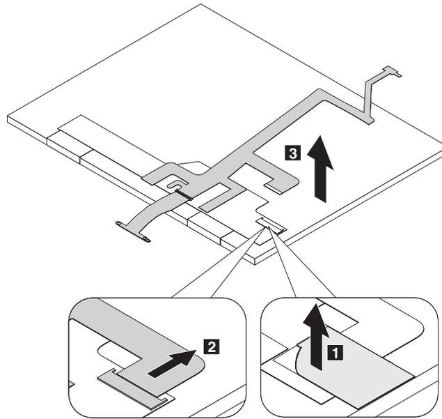
**When installing:** Make sure that the cable is positioned correctly, the connector is attached firmly, and the tape is reattached.
