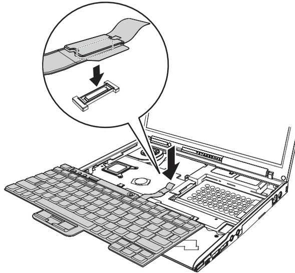
2. Make sure that the keyboard edges are under the frame. Then press the keys to latch the keyboard firmly in place.
