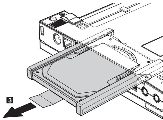
**When installing:** Make sure that the hard disk is connected firmly.
