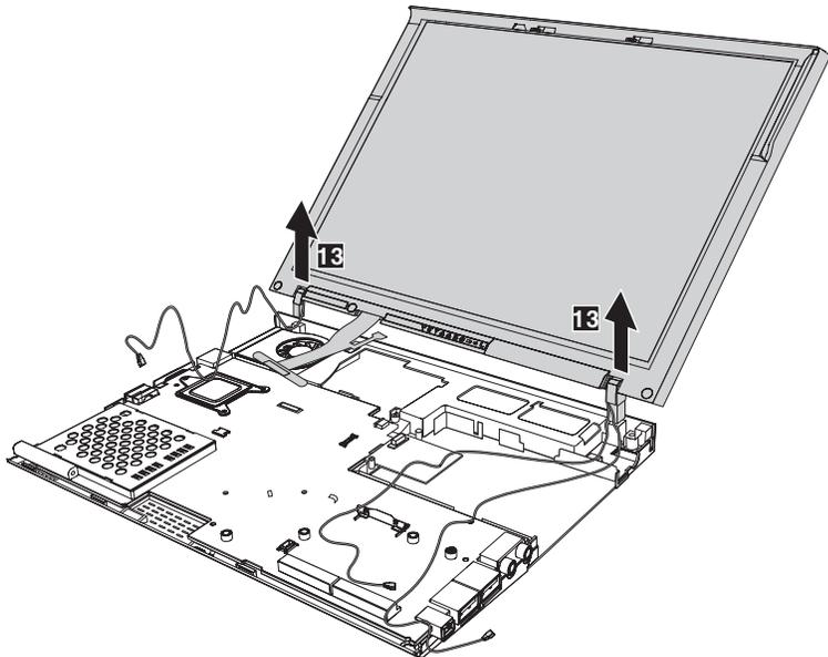
**When installing:** When fitting the LCD hinge into the system, make sure the wireless antenna cables do not get pinched in by the hinge. Then route the wireless antenna cables as shown below. For wireless WAN: red is main; blue is aux. For wireless LAN: gray is main; black is aux. Remember to reattach the mylar and tapes.
