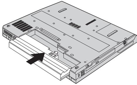
5. Slide the battery latch to the lock position.
