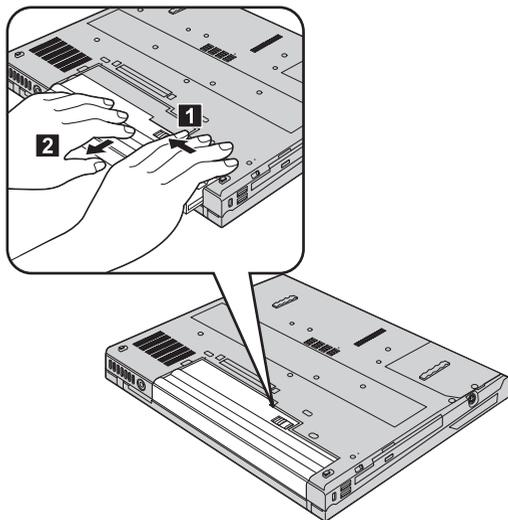
4. Align the front of a fully charged spare battery with the front side of the battery space in the computer; then gently push the battery into the space.
