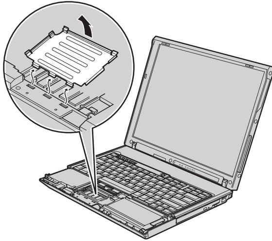
9. If two SO-DIMMs are already installed in the memory slot, remove one of them to make room for the new one by pressing out on the latches on both edges of the socket at the same time **1**. Be sure to save it for future use **2**.
