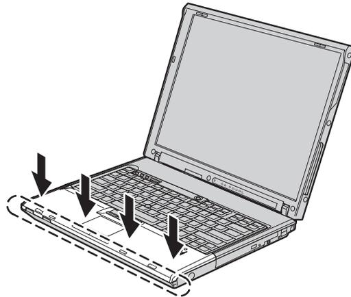
16. Close the computer display, and turn the computer over; then replace the screws that secure the palm rest.
