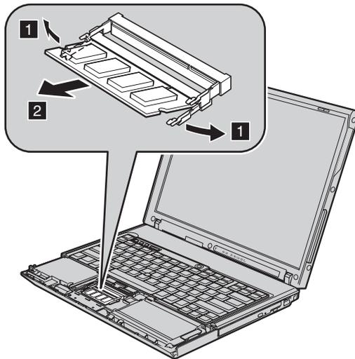
10. With the notched end of the SO-DIMM toward the contact edge side of the socket, firmly insert the SO-DIMM into the socket at an angle of about 20 degrees **1**; then pivot it downward until it snaps into place **2**.
