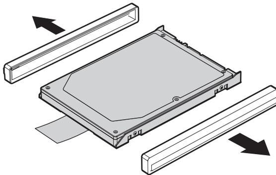
7. Attach the side rubber rails to a new hard disk drive.
