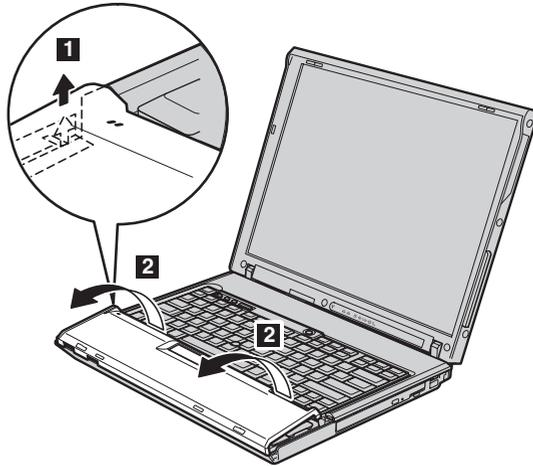
**Note:** When you lift the left and front edges of the palm rest, it is normal to hear a click.
