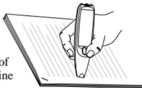
3. Move C-Pen over the line of text. Keep the pen tip flat against the surface while reading. Make sure the autotrigger (at the pen tip) is pressed backwards into the pen.
