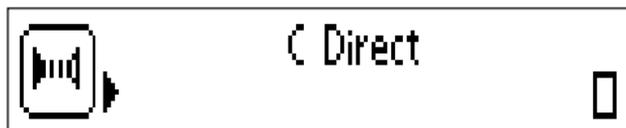
When you read text now with C-Pen, it will appear as usual on the display. To transfer the text to the active application in Windows, direct C-Pen’s IR-eye towards the IR port of the PC. The text will disappear from C-Pen’s display and be transferred to the cursor position in the active Windows application.
