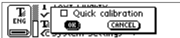
**Quick calibration** enables C-Pen to start a calibration as soon as you press **Trigg** and hold the pen still for about two seconds. **Quick calibration** is a preferred option if you often read texts with very different text contrasts. **Quick calibration** is disabled as default.
