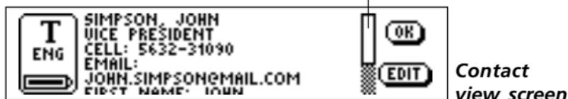
To select **OK** or **EDIT**, first press **Nav** to deactivate the scroll bar – the rectangle stops blinking – then turn **Nav** to go to the buttons.
