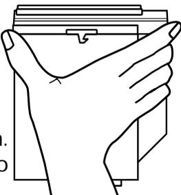
**5** Insert the VST Zip Drive in the UltraSlimBay until it is connected firmly.
