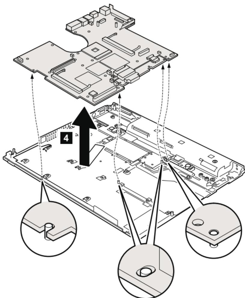
**When installing:** Make sure that the all the guide holes of the system board are firmly attached to the base cover.
