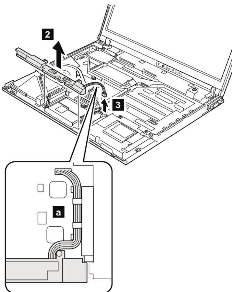
**When installing:** Make sure that the connector **3** is firmly attached. Then route the cable as in **a**.
