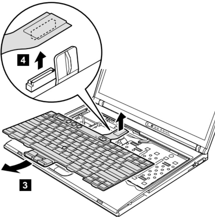
**When installing:** Make sure that the connector **4** is firmly attached.
