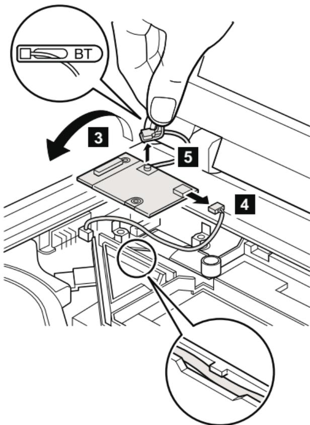
**When installing:** Make sure that connector **4**, the jack **5**, and the connector on the underside of the card are firmly attached. Then place the cable to fit in the cable guide as in the figure.
