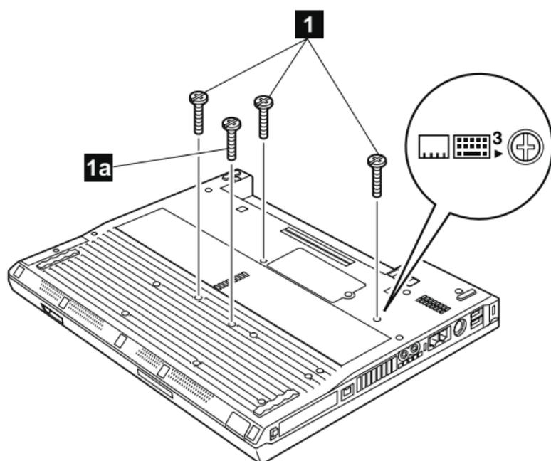
Screw **1a** is only for the models with 14.1-in. LCD.
