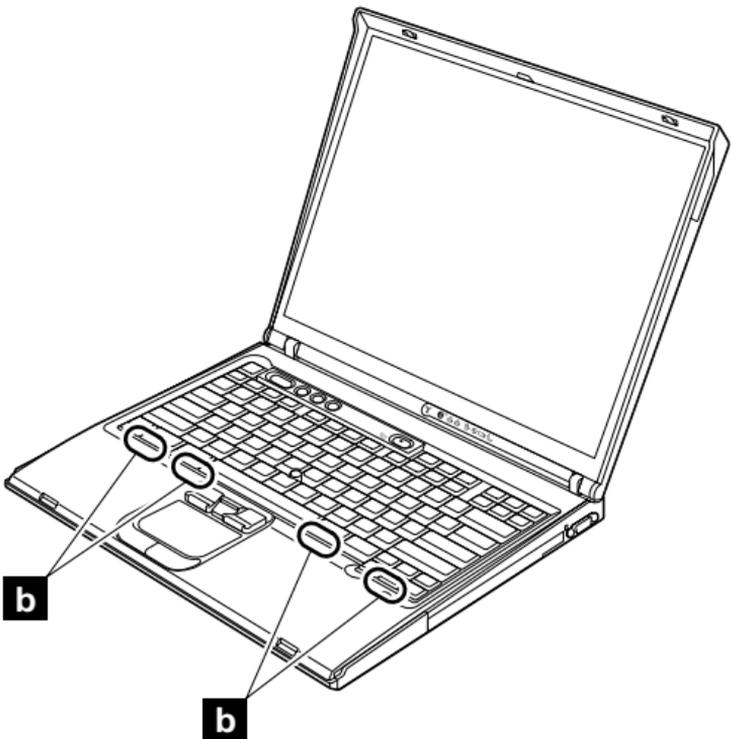
5. Secure the keyboard from the underside of the computer, using the new screws provided with the keyboard.
