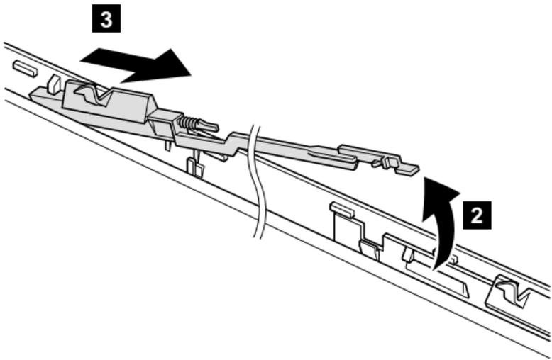
**When installing:** Attach the left latch to the LCD cover as in this figure.
