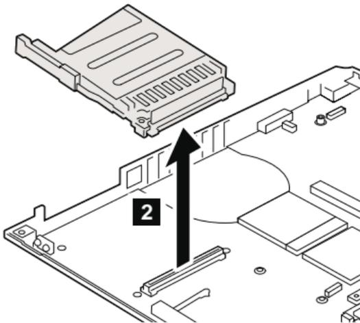
**When installing:** Make sure that the connector **2** is firmly attached to the system board. Then, secure the screws from the underside of the computer.
