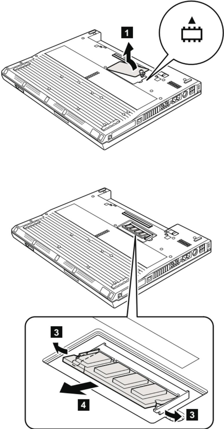
**When installing:** Insert the notched end of the DIMM into the socket. Press the DIMM firmly, and pivot it until it snaps into the place. Make sure that it is firmly fixed in the slot and does not move easily.
