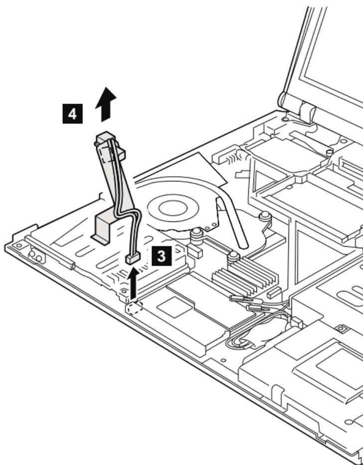
Remove the connector **3**. And strip the tape securing the IEEE 1394 cable to the PC Card slot and remove the IEEE 1394 cable **4**.
