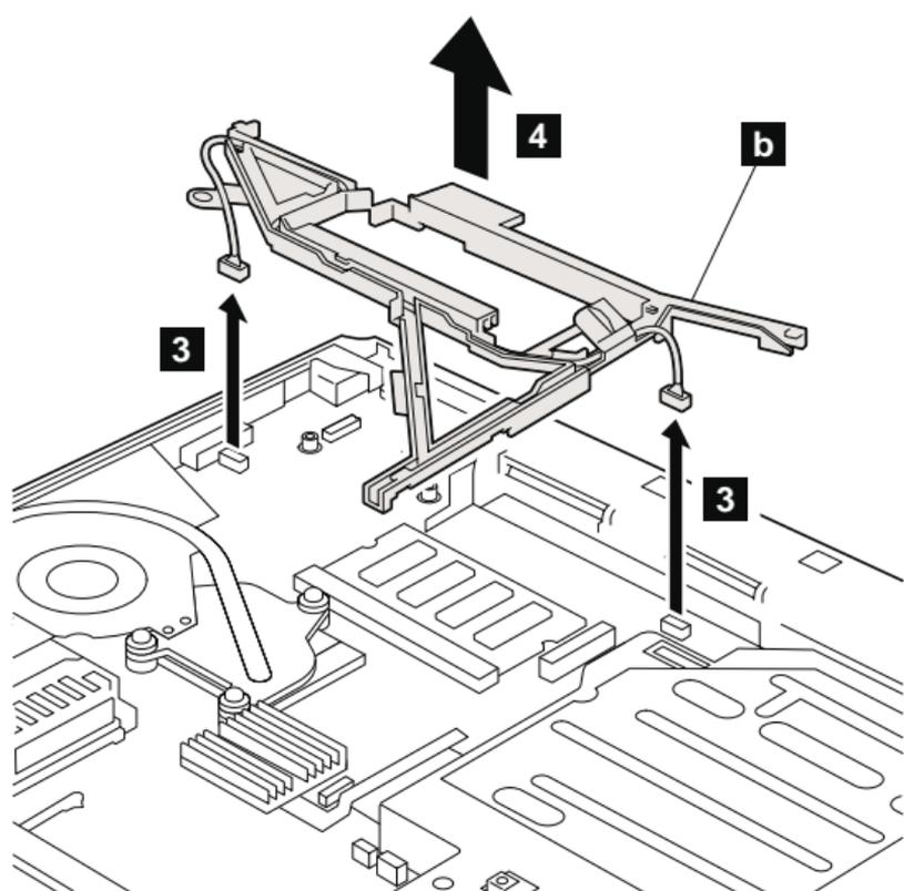
**When installing:** Make sure that the connectors **3** are firmly attached.
