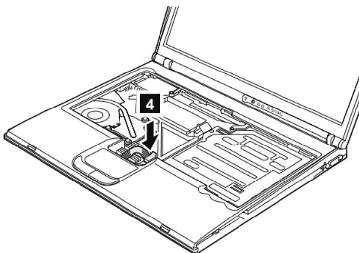
4. Secure the keyboard bezel from the underside of the computer with the screws.
