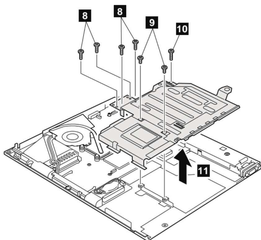
Screws **8** are only for the models with 15.0-in. LCD. For the other models, skip the step.
