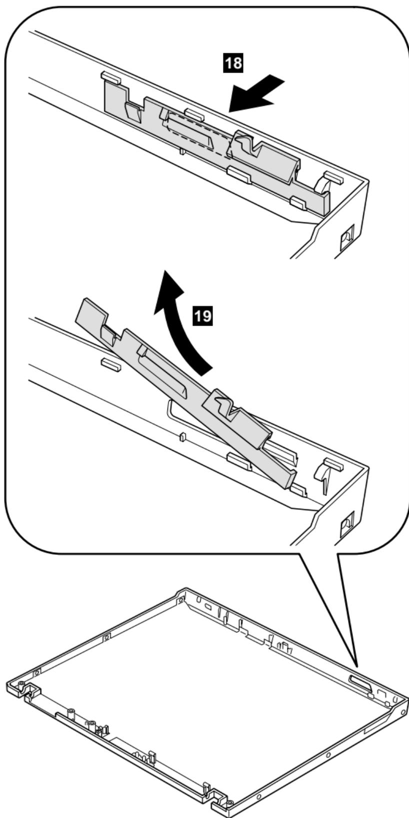
**When installing:** Attach the right latch to the LCD cover as in this figure.
