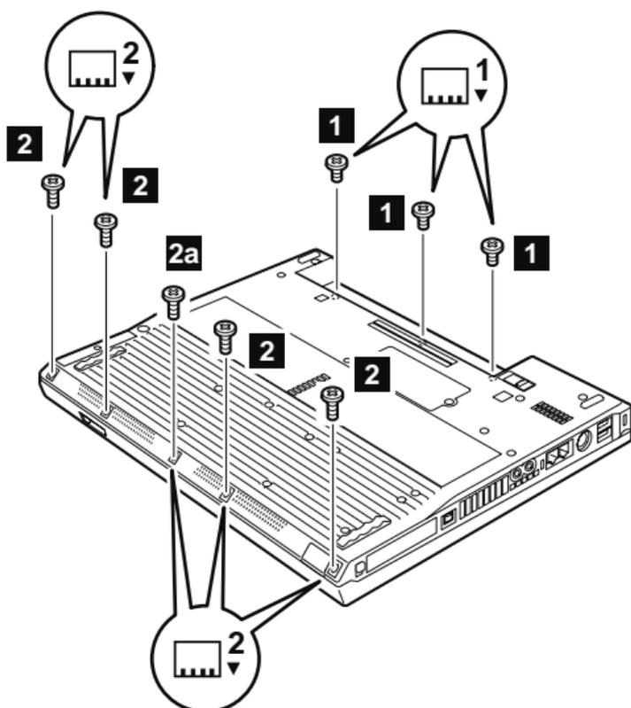
Screw **2a** is only for the models with 15.0-in. LCD.
