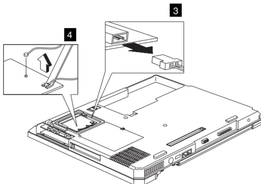
**Note:** There are 2 cables on step 4 : The gray cable is the main antenna and the black cable is the auxiliary antenna.
