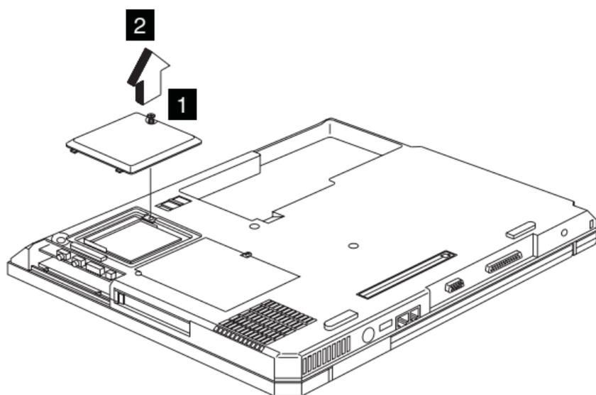
**Note:** The screw does not separate from the PCI cover.
