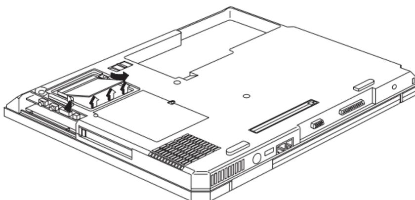
**Note:** When you install the PCI card, remember to press it down and ensure the connection is well.
