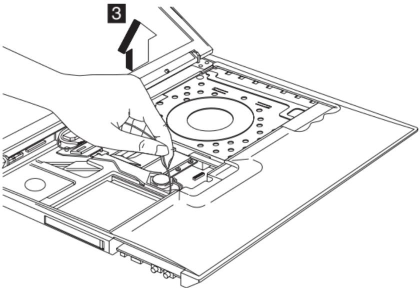
**Note:** Release the gray cable, which is the main antenna from the system.
