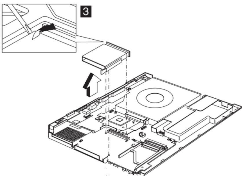
**Note:** Before removing and replacing the PCMCIA holder, make sure that the PCMCIA cards are removed and the eject levers are sticking out.
