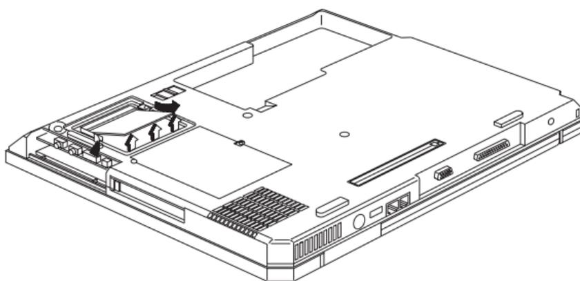
**Note:** When you install the PCI card, remember to press it down and ensure the connection is well.
