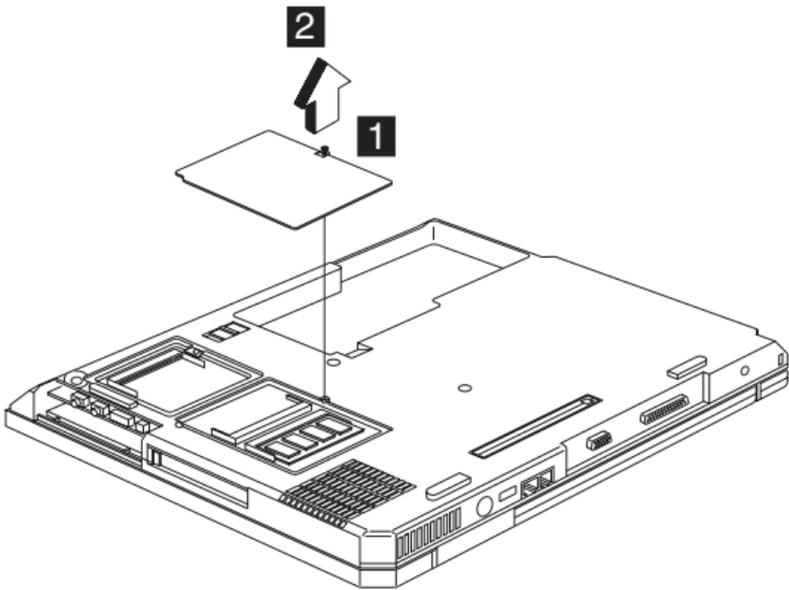
**Note:** The screw does not separate from the memory cover.
