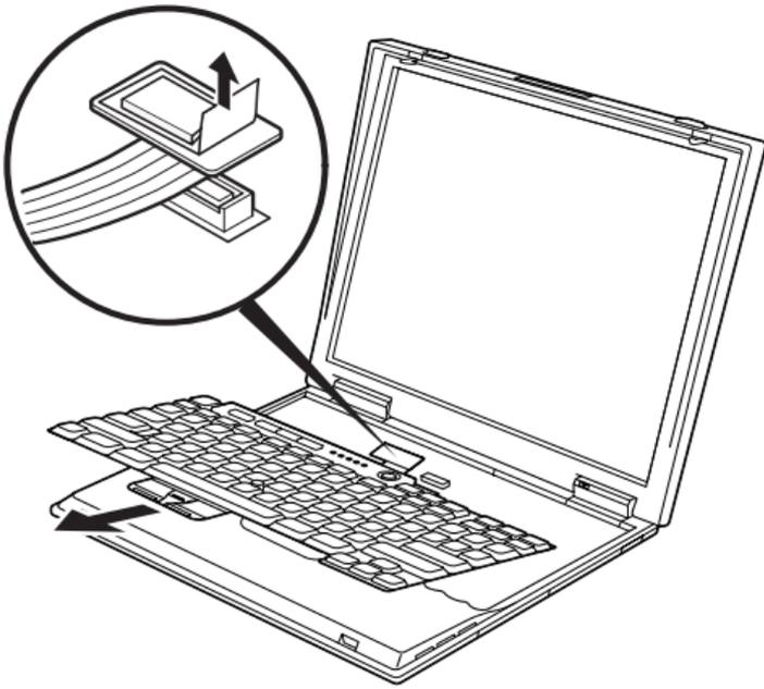
When installing: When installing the keyboard, do as follows:
