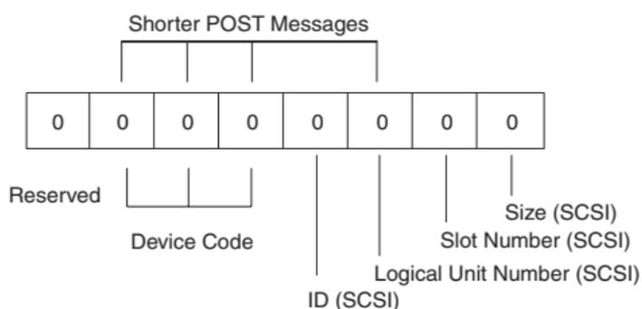
Each SCSI device is assigned a unique SCSI ID. Duplicate SCSI ID settings can generate a false error message. Use the SCSI ID to determine whether an error message is coming from an internal or an external device.
