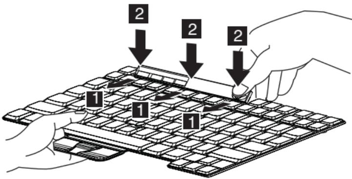
1. Align the KBD Control Panel hooks with the corresponding slots like the picture.
