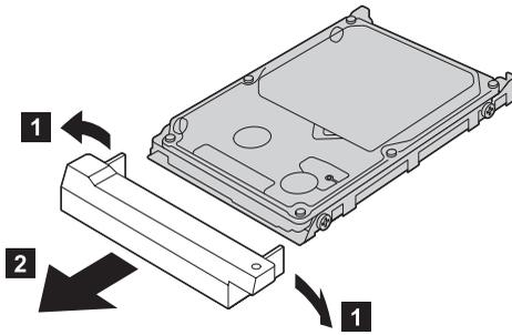
7. Attach the cover to a new hard disk drive.
