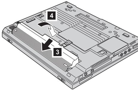
5. Slide the battery latch to lock it.
