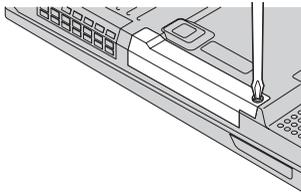
5. Remove the hard disk drive by pulling the cover away from the computer.
