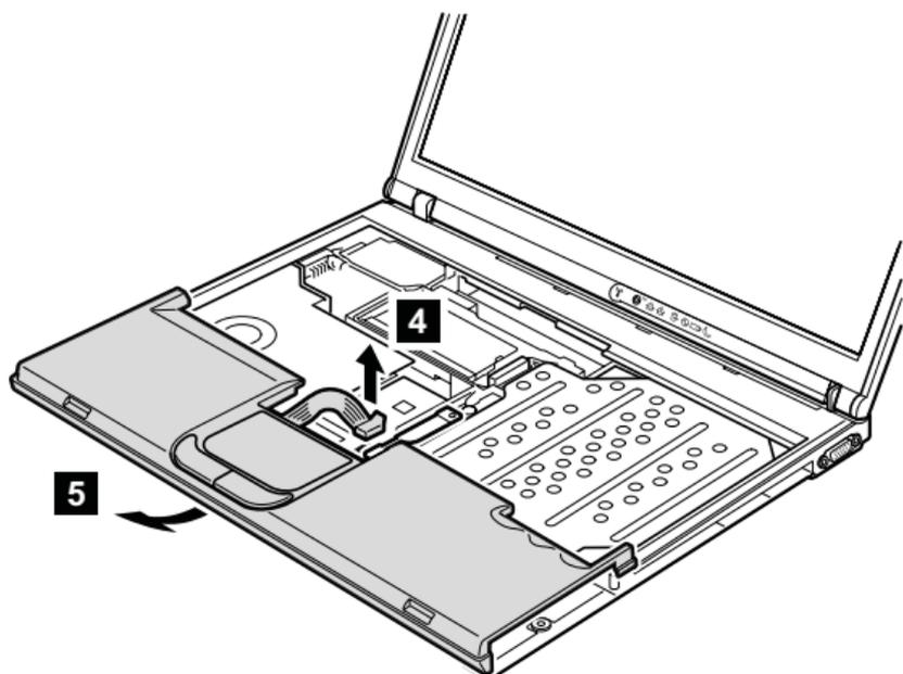
**When installing:** On a model with a touch pad, make sure that connector **4** is firmly attached.
