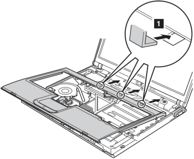
While inserting the three latches, align the top-left corner of the keyboard bezel as in figure **a**.
