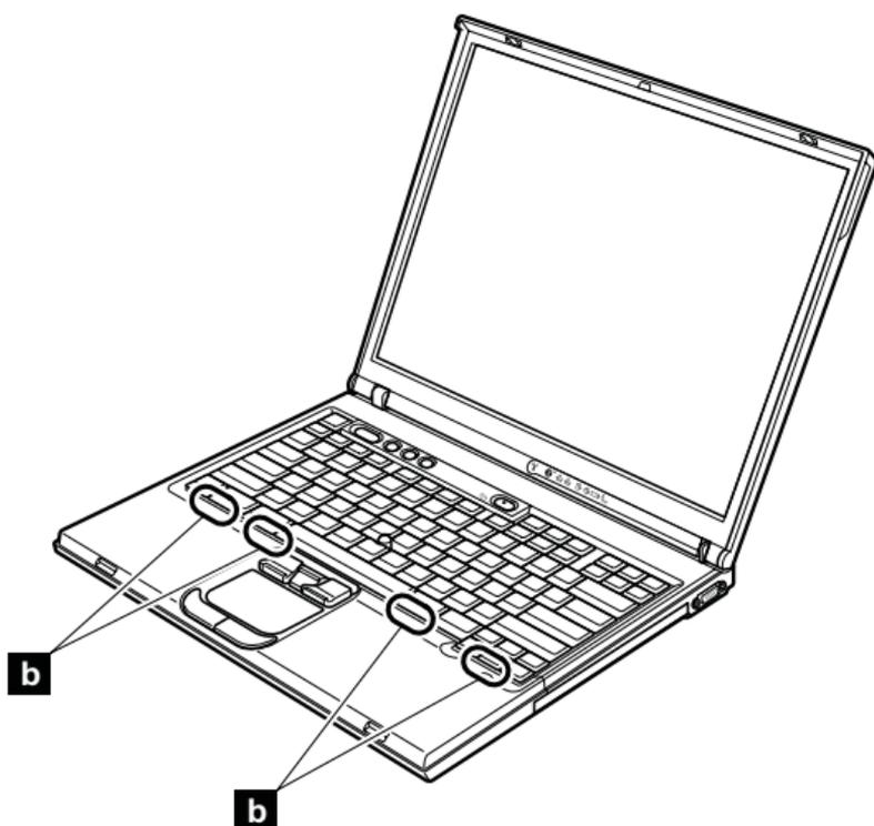
5. Secure the keyboard from the underside of the computer, using the new screws provided with the keyboard.
