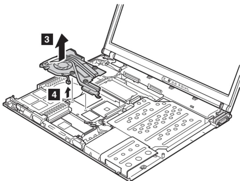
**When installing:** Make sure that the connector **4** is firmly attached.
