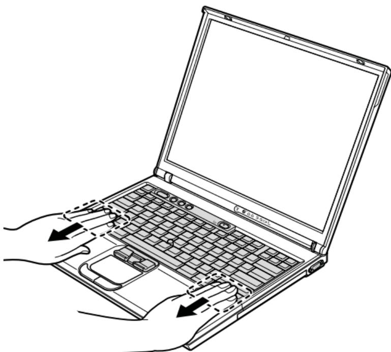
4. Make sure that all the projections on the front side of the keyboard **b** are firmly attached under the frame.
