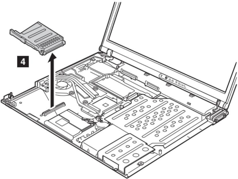
**When installing:** Make sure that the connector on the underside of the PC card slot **2** is firmly attached, and then secure the slot with the screws.
