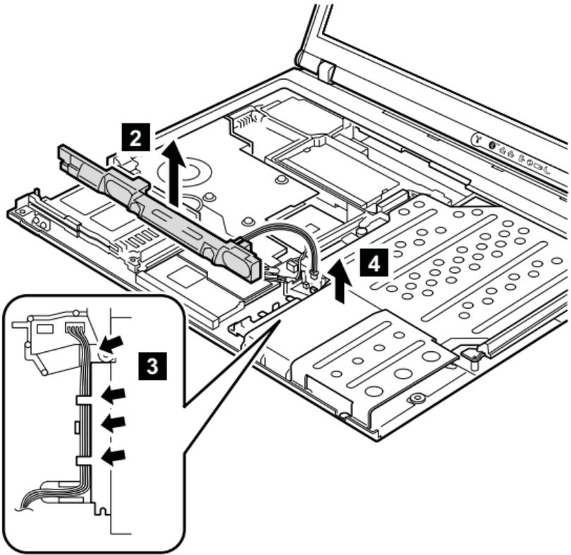
**When installing:** Make sure that the connector **4** is firmly attached. Then route the cable as in **3** .
