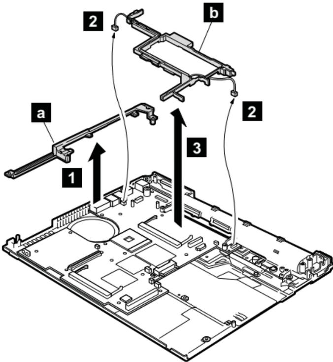
**When installing:** Make sure that the connectors **2** are firmly attached to the system board.
