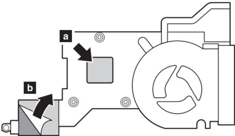
Figure 2. Fan assembly, long
