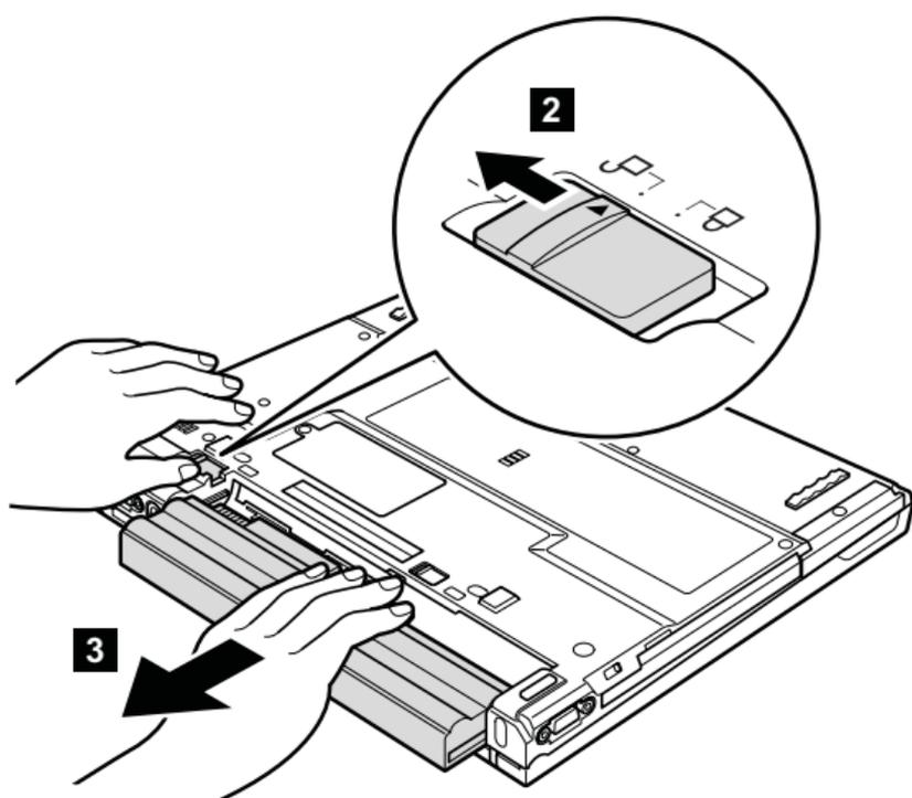
**When installing:** Install the battery pack along the slide rails on the left and right sides of the battery-pack slot. Then make sure that both battery latches, **a** and **b**, are locked, as in the following figure.
