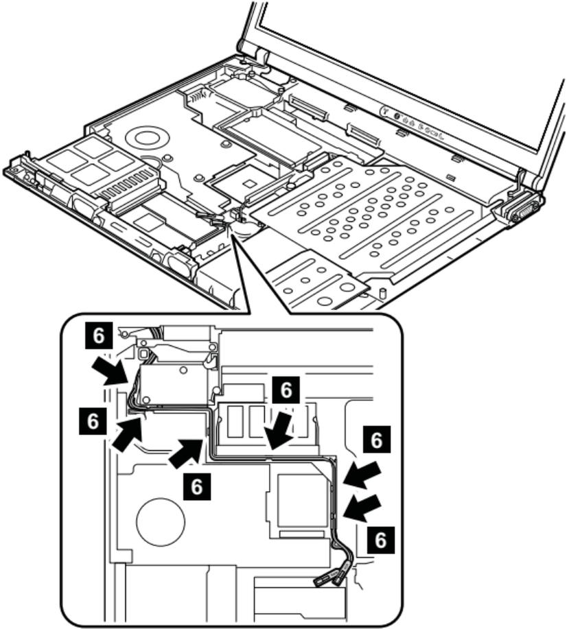
**When installing:** Make sure that the antenna cables are correctly routed and securely in place.
