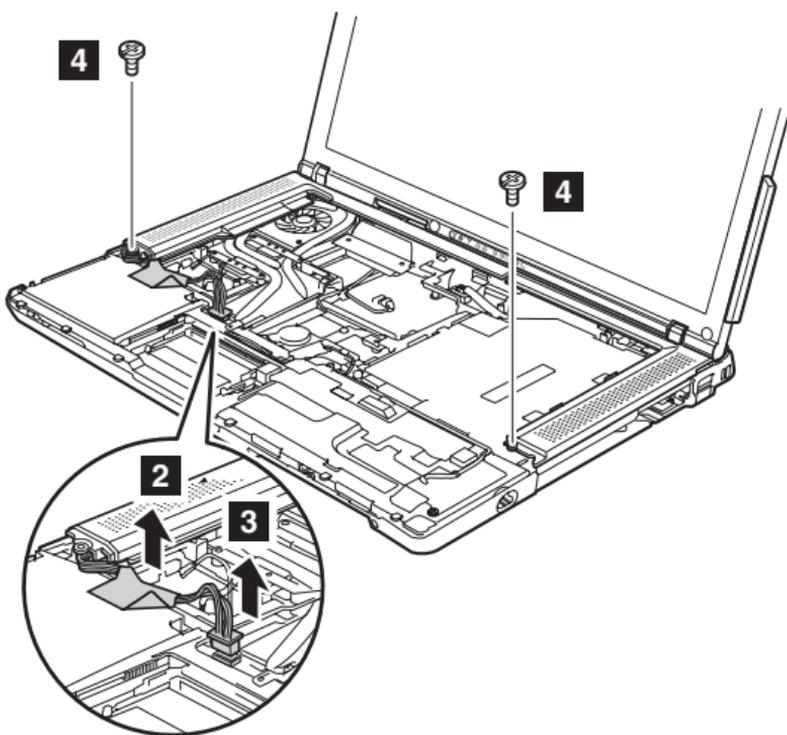
Strip the tape that secures the cable **2**, and disconnect the speaker cable **3**.
