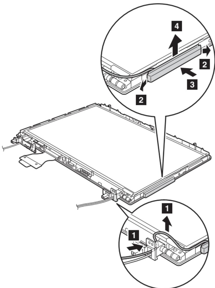
**When installing:** In step **2**, press the part indicated by the arrow until it snaps into place.
