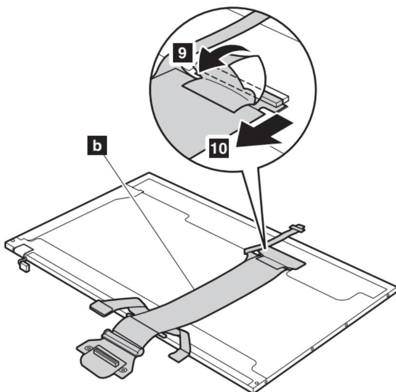
**When installing:** When replacing any LCD FRUs, be sure not to pinch the antenna cables. Make sure that the cables are routed as shown in the figures on page 133 and 134.
