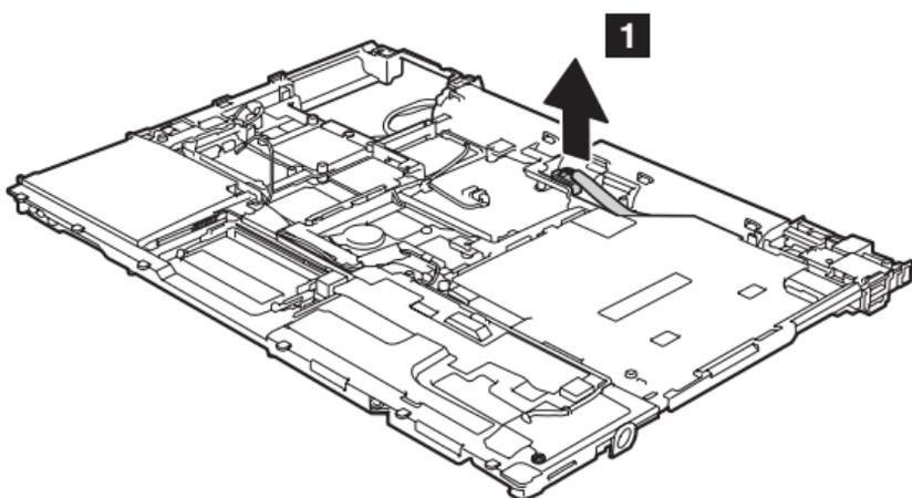
**When installing:** Make sure that the connector **1** is attached firmly.
