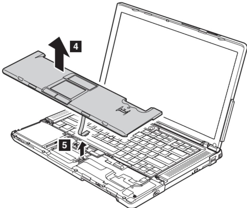
**When installing:** Make sure that the touch pad connector is attached firmly.
