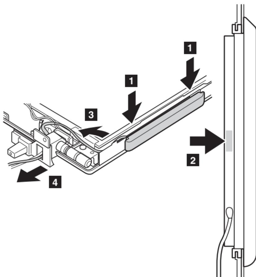
**Note:** In step **4**, do not tense the cable. To do so, the cable may get damaged by the hinge, and may cause a broken wire.
