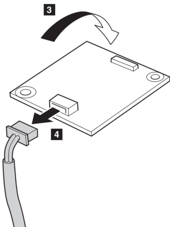
**When installing:** Make sure that the modem connector and the connector on the underside of the card are attached firmly.
