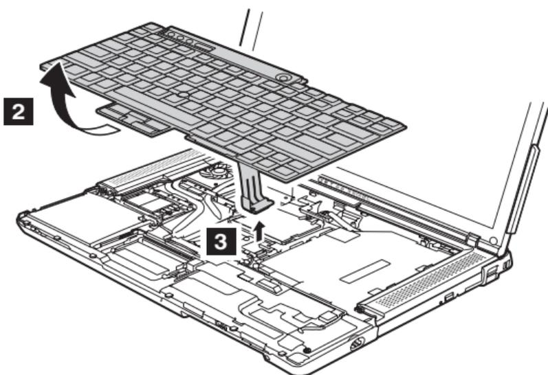
**When installing:** Make sure that the keyboard edges **a** are under the frame as shown in this figure.
