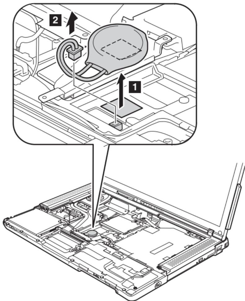
**When installing:** Make sure that the battery connector is attached firmly.
