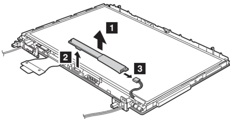
**When installing:** Make sure that connectors **2** and **3** are attached firmly.
