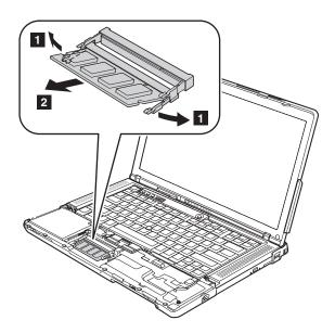
When installing: Insert the notched end of the DIMM into the socket. Press the DIMM firmly, and pivot it until it snaps into the place. Make sure that it is firmly fixed in the slot and does not move easily.
