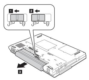
**When installing:** Install the battery pack along the slide rails of the slot. Then make sure that the battery release lever is locked, as in this figure.
