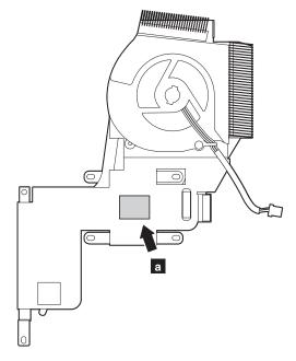
• Make sure that the fan connector is attached firmly. (continued)
