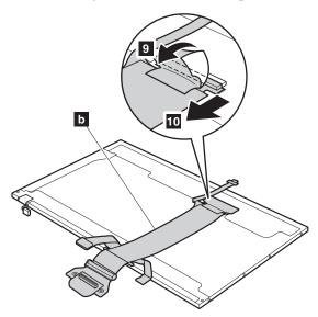
When installing: When replacing any LCD FRUs, be sure not to pinch the antenna cables. Make sure that the cables are routed as shown in the figures on page 117 and 118.
