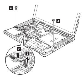
Strip the tape that secures the cable **2**, and disconnect the speaker cable **3**.
