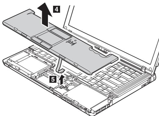
**When installing:** Make sure that the touch pad connector is attached firmly.
