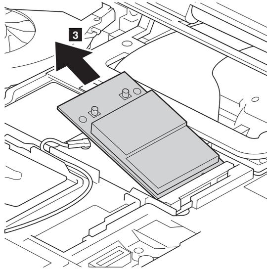
**When installing:** Plug the red cable into the jack labeled **MAIN** on the card, and the blue cable into the jack labeled **DIV**.
