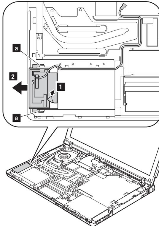
**When installing:** Make sure that the antenna cable is routed along the cable guides, and that the antenna is attached to the guides **a** firmly.
