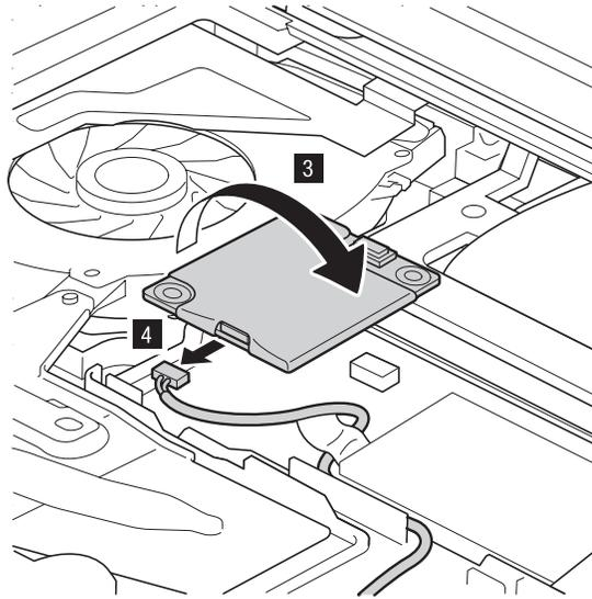
**When installing:** Make sure that the modem connector and the connector on the underside of the card are attached firmly.
