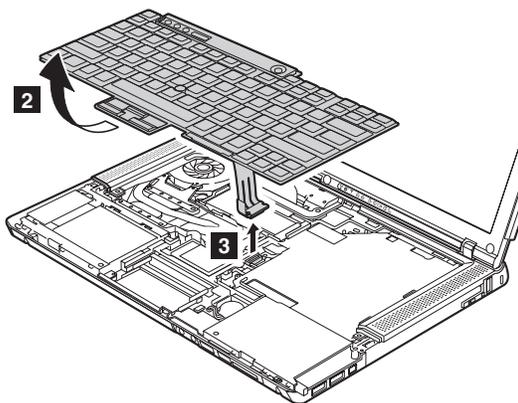
**When installing:** Make sure that the keyboard edges **a** are under the frame as shown in this figure.
