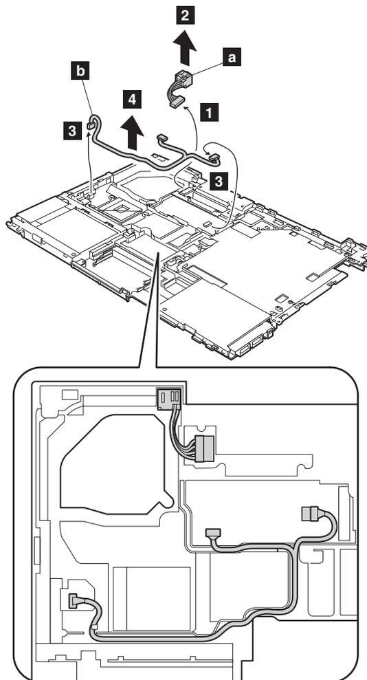
**When installing:** Make sure that the connectors **1** and **3** are attached firmly, and that the cables are routed as in the figure above.
