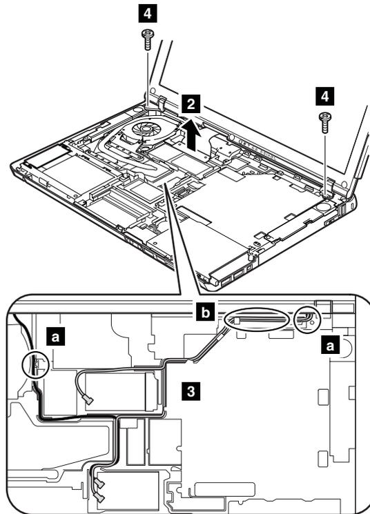
In step **3**, release the antenna cables from the cable guides.
