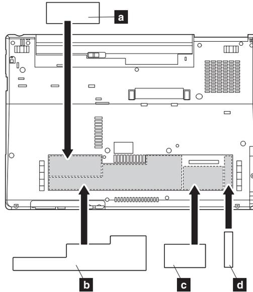
For some models, you also need to apply one or two FCC labels or the other types of labels. Check the old base cover; if it has one or two FCC labels or the other types of labels, find duplicates of them in the package and apply them to the new base cover.
