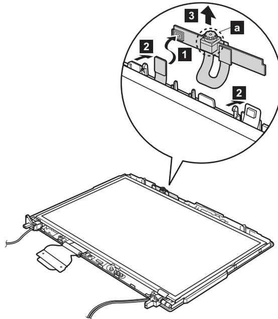
**Note:** The part marked **a** is fragile and easy to break. When you deal with the camera assembly, do not hold that part to avoid damage.
