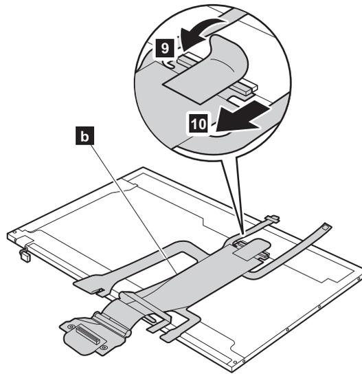
**When installing:** When replacing any LCD FRUs, be sure not to pinch the antenna cables. Make sure that the cables are routed as shown in the figures on page 113 and 114.
