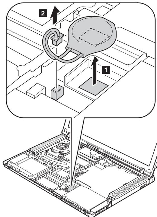
**When installing:** Make sure that the battery connector is attached firmly.
