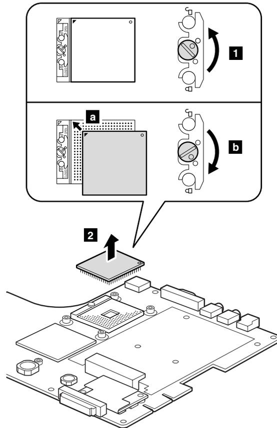
**When installing:** Place the CPU on the CPU socket **a**, and then rotate the head of the screw in the direction shown by arrow **b** to secure the CPU.
