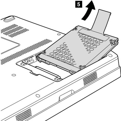
**When installing:** Make sure that the hard disk drive connector is attached firmly.
