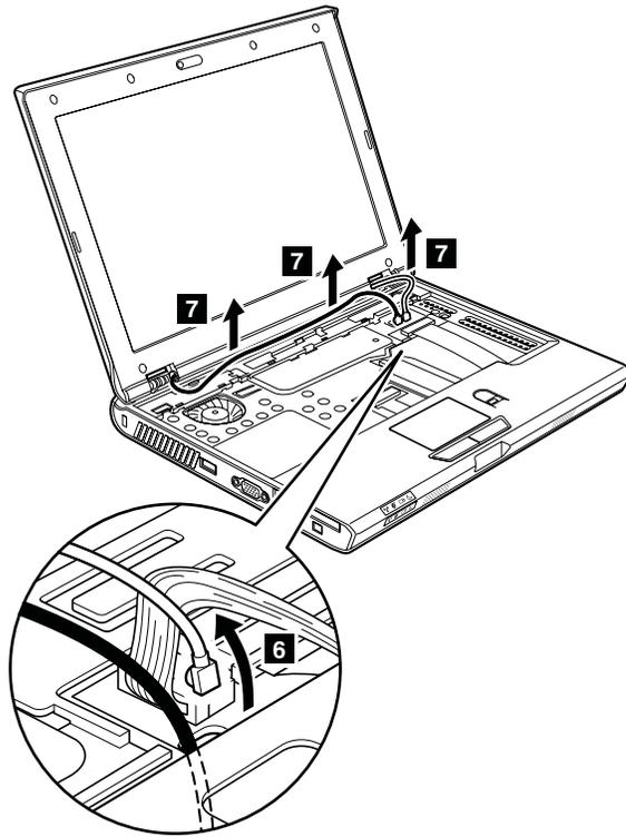
**When installing:** Route the antenna cables along the cable guides. When you route the cables, do not tense them. To do so, the cables may get damaged by the cable guides of the frame, and may cause a broken wire.
