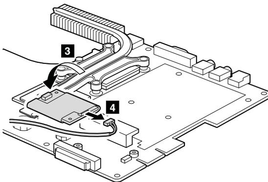
**When installing:** Make sure that the connector on the underside of the card is attached to the system board firmly, and then fasten the screws.
