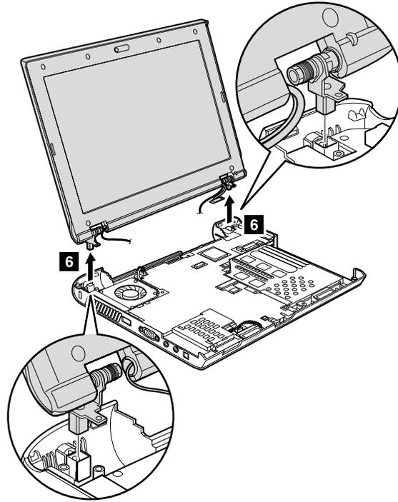
**When installing:** When you attach the LCD unit, make sure that you do not pinch the antenna cable.
