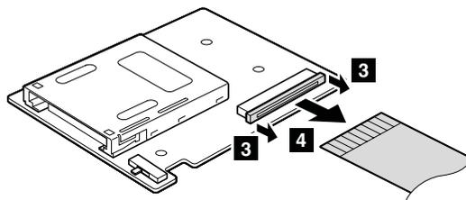
**When installing:** Make sure that all the connectors are attached firmly.
