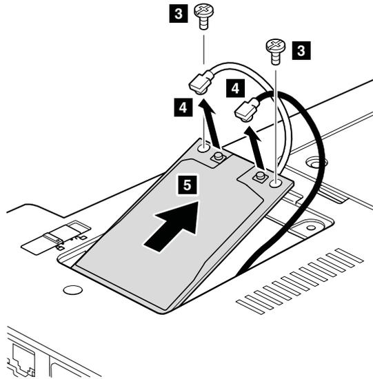
In step **2**, unplug the jacks by using the removal tool antenna RF connector (P/N: 08K7159) or pick the connectors with your fingers and gently unplug them in direction of the arrow.
