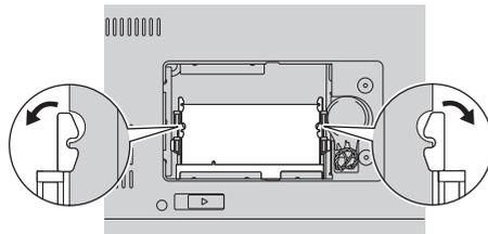
7. Find the notch on the contact edge side of the SO-DIMM.
