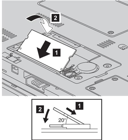
9. Push the SO-DIMM down until it snaps into place.
