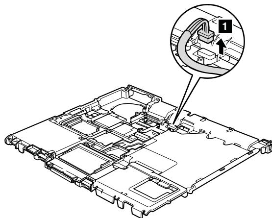
**When installing:** Make sure that the connector **1** is attached firmly.
