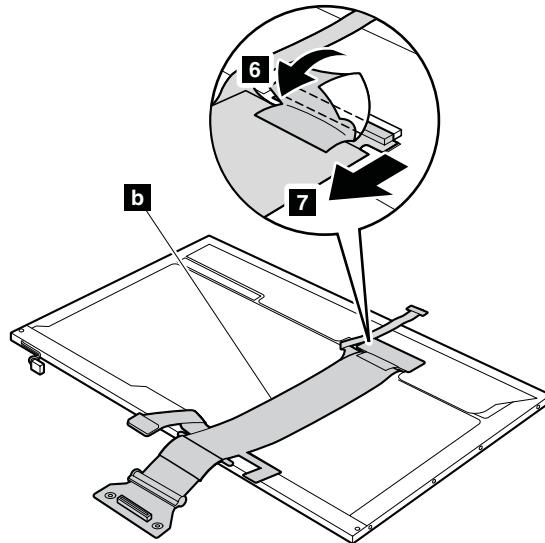
**When installing:** When attaching the LCD panel, be sure not to pinch the antenna cables, and make sure that the cables are routed as shown in these figures.
