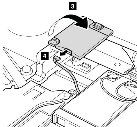
**When installing:** Make sure that the modem connector and the connector on the underside of the card are attached firmly.
