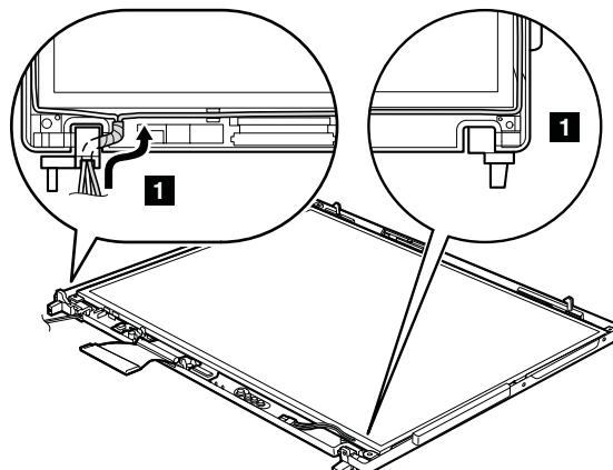
**When installing:** When routing the antenna cable, do not tense the cable. To do so, the cable may get damaged by the hinge, and may cause a broken wire.
