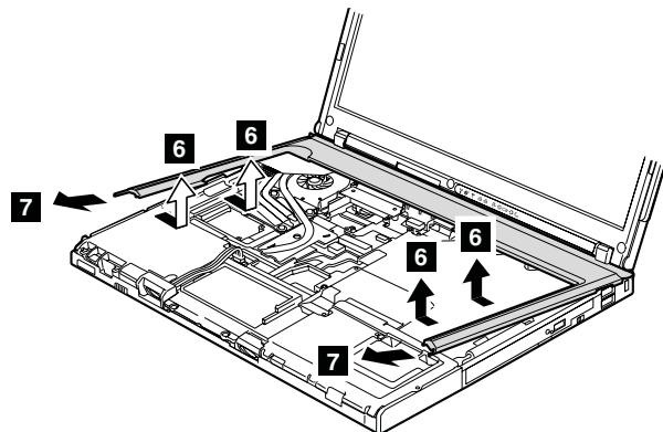
**When installing:** Make sure that all the claws are attached firmly. Then fasten the screws to secure the keyboard bezel.
