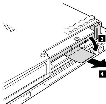
**When installing:** Make sure that the hard disk drive connector is attached firmly.
