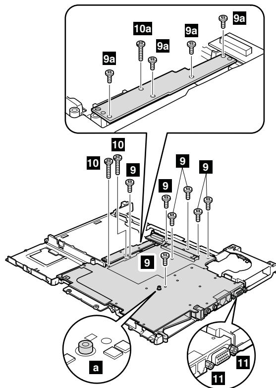
**Note:** Screws **9a** and **10a** are only for the models with 15.0-in. LCD.
