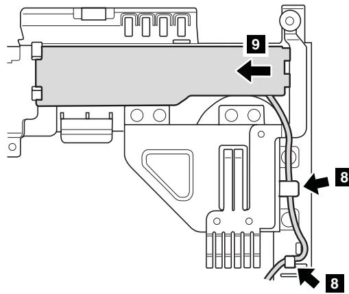
**When installing:** Make sure that the antenna cable is routed along the cable guides.
