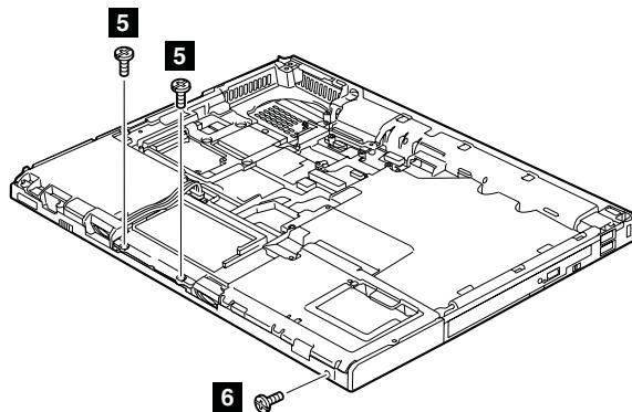
**Note:** Screw **6** is only for the 14.1-in. LCD models.
