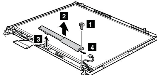
**Note:** Step **1** is only for the models with 14.1-in. LCD. Inverter card in the models with 15.0-in. LCD does not have the screw **1**.
