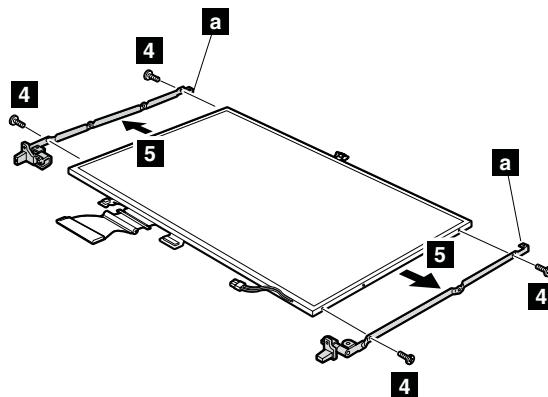
Remove the hinges ( **a** ) from the LCD panel.
