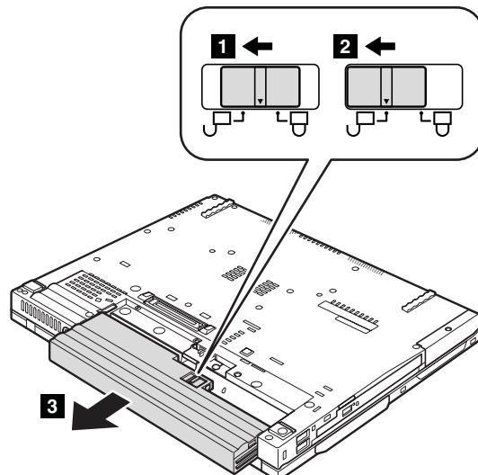
**When installing:** Install the battery pack along the slide rails of the slot. Then make sure that the battery release lever is in the locked position as in this figure.
