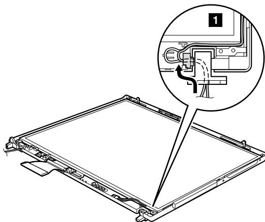
**When installing:** As you route the cables, make sure that they are not subjected to any tension. Tension could cause the cables to be damaged by the cable guides, or a wire to be broken.
