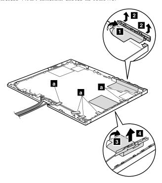
**Cable routing:** When you attach the antenna cables, route the cables as shown in this figure.
