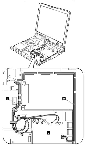
When installing: Make sure that the cables are routed as shown in this figure. (continued)
