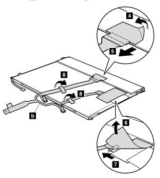
**When installing:** Make sure that the connectors of the LCD cable are attached firmly.
