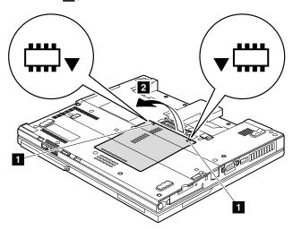
Remove the DIMM as shown in this figure.
