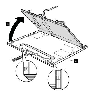
**When installing:** Place the FFC ( a ) on the rear cover of the LCD, in the direction shown in the figure above.
