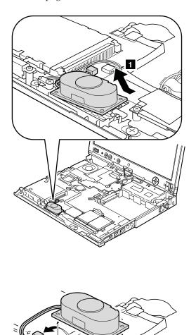
When installing: Make sure that the speaker connector is attached firmly.
