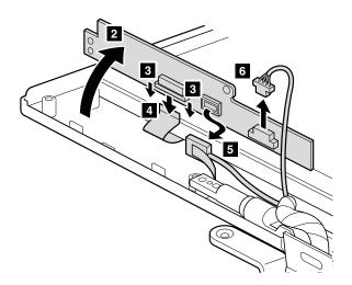
When installing: Make sure that connectors [4], [5], and [6] are attached firmly.
