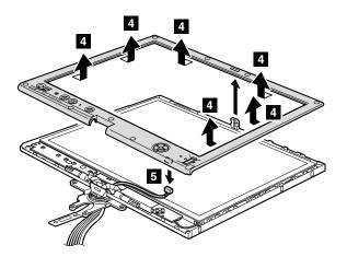
When installing: Make sure that the connector is attached firmly.
