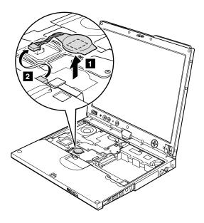
When installing: Make sure that the battery connector is attached firmly.
