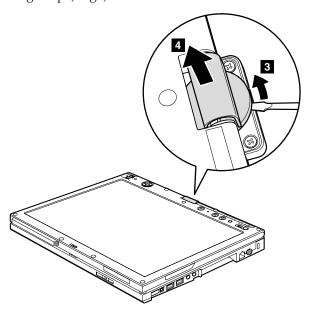
Before removing the hinge cap (small) in step  $\fill 5$ , rotate the LCD unit back to the original position, and close the LCD cover.
