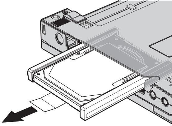
6. Detach the side rubber rails from the hard disk drive.
