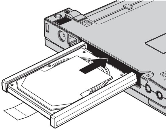
9. Reinstall the cover of the hard disk drive slot **1**. Then, reinstall the screw **2**.
