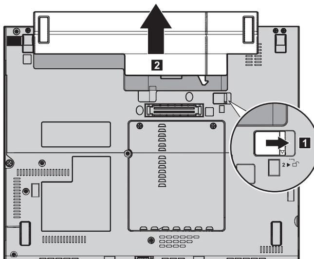
5. Install a fully charged battery.
