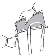
Use a quality carrying case that provides adequate cushion and protection. Do not pack your computer in a tightly packed suitcase or bag.
