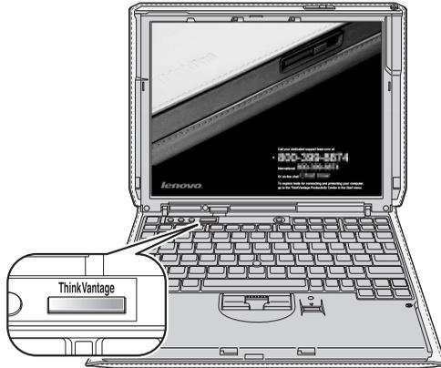
**Note:** You can also use the ThinkVantage button to interrupt the startup sequence of your computer and start the Rescue and Recovery™ workspace, which runs independently of the Windows operating system and is hidden from it.
