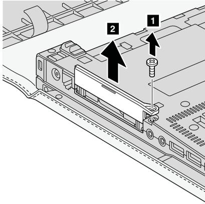
6. Remove the hard disk by pulling out the tab.
