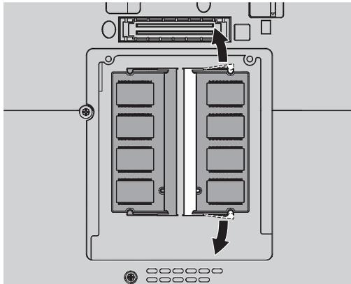
8. With the notched end of the SO-DIMM toward the contact edge side of the socket, firmly insert the SO-DIMM into the socket at an angle of about 20 degrees **1**; then pivot it downward until it snaps into place **2**.
