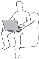
When your computer is turned on or the battery is charging, the base, the palm rest, and some other parts may become hot. Avoid keeping your hands, your lap, or any other part of your body in contact with a hot section of the computer for any extended length of time. When you use the keyboard, avoid keeping your palms on the palm rest for a prolonged period of time.
