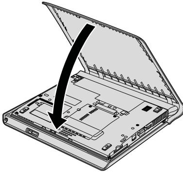
2. While holding the front side of the computer as shown in the drawing, pull the cover toward you and downward.
