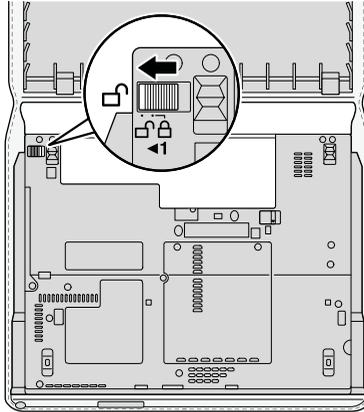
4. Slide and hold the battery latch **1**. Then, remove the battery **2**.
