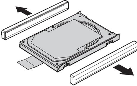
8. Attach the side rubber rails to a new hard disk drive.
