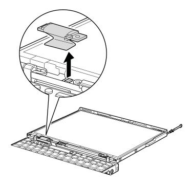
When installing: Make sure that the connector is attached firmly.
