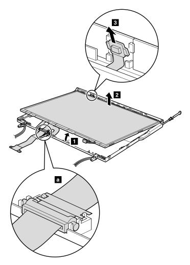
When installing: Make sure that the LCD cable and the cable guide are attached firmly as shown in a.
