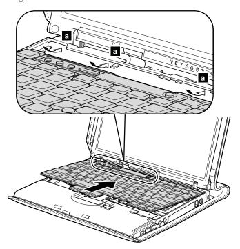
3. To make sure that the front side of the keyboard is housed firmly, gently press the keys with your thumbs and try to slide the keyboard toward you.
