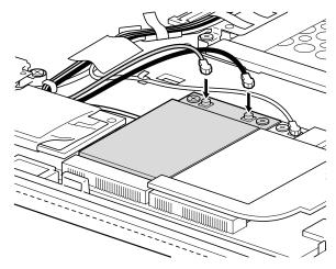
3. If the computer you are servicing has three cables and the card has three connectors, plug the gray cable (MAIN) into the jack labeled **TR1**, the white cable (3rd) into jack labeled **R0**, and the black cable (AUX) into jack labeled **TR2** on the card.
