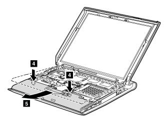
When installing: Make sure that the claw is attached firmly front edge of the keyboard bezel 2.
