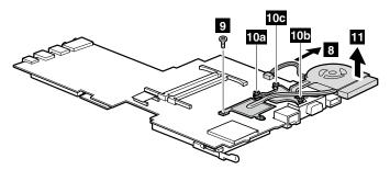
Note: Remove the fansink screws in the order shown 10a, 10b, and 10c.
