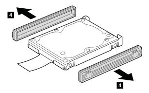
**When installing:** The rubber rails on the hard disk drive must be attached to the replacement drive. Otherwise the drive cannot be installed properly.
