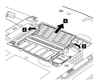
When installing: Insert the notched end of the DIMM into the socket. Press the DIMM firmly, and pivot it until it snaps into the place. Make sure that it is firmly fixed in the slot and does not move easily.
