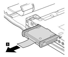
When installing: Make sure that the hard disk drive connector is attached firmly.
