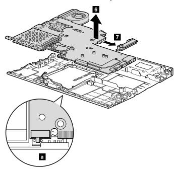
When installing: When attaching the system board to the base cover, adjust the placement of the wireless radio switch as shown in a .
