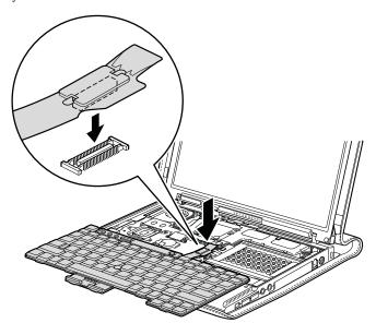
2. Attach the keyboard so that the keyboard edges **a** are under the frame as shown in this figure.
