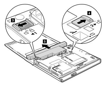
**When installing:** Install the battery pack along the slide rails of the slot. Then make sure that the battery release lever is in the locked position.
