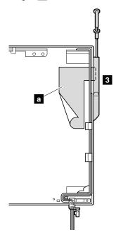
**When installing:** As you route the cables, make sure that they are not subjected to any tension. Tension could cause the cables to be damaged by the cable guides, or a wire to be broken.
