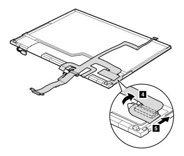
When installing: Make sure that the LCD cable is attached firmly.
