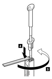
In step 5, detach the rod antenna from the antenna cable.
