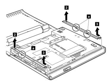
**When installing:** Make sure that the latches on the bottom side of each bezel are attached firmly.
