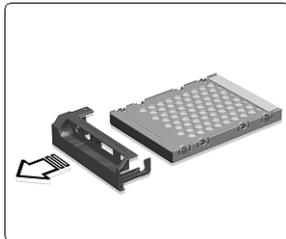
7. Attach the cover to a new hard disk drive.
