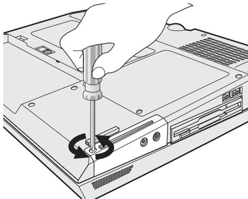
5. Open the computer display; then stand the computer on its side and remove the hard disk drive by pulling the cover away from the computer.
