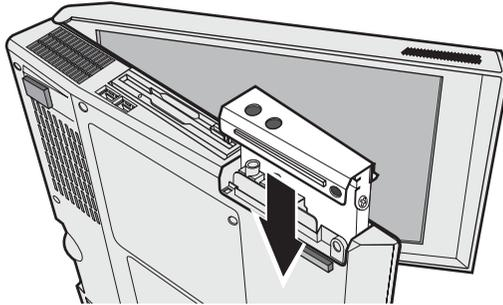
9. Turn the computer over so that its bottom side is up. Reinstall the screw.
