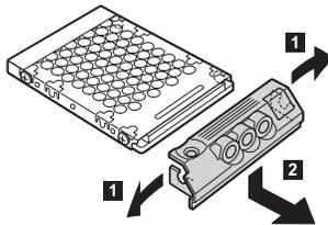
7. Attach the cover to a new hard disk drive.
