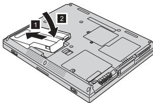
5. Slide the battery latch to the left to lock it.
