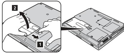
4. Align the side of a fully charged spare battery with the side of the battery space in the computer **1**; then gently push the battery into the space **2**.
