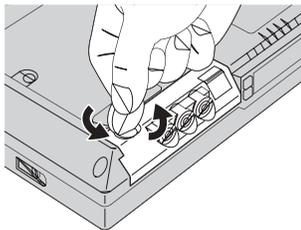
5. Open the computer display; then stand the computer on its side and remove the hard disk drive by pulling the cover away from the computer.
