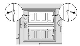
**5.** Find the notch on the side of the SO-DIMM.
