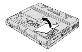
If the SO-DIMM is already in the memory slot, remove it to make room for the new one by pressing out on the latches on both edges of the socket at the same time. Be sure to save it for future use.
