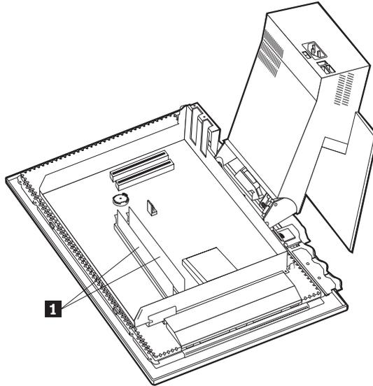
4. Locate the DIMM sockets on the system board. See “System board” on page 39.
