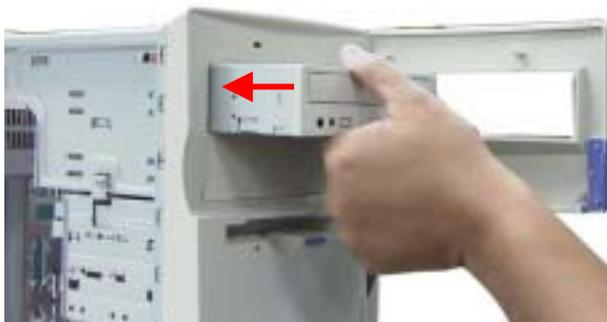
**5.** Slide the CD-ROM drive into the bay and align the drive's faceplate with the front of the case.
