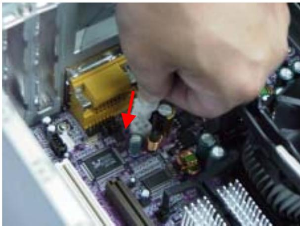
**5.** Connect the +12V power connector. Make sure the power connectors are properly seated and firmly attached.
