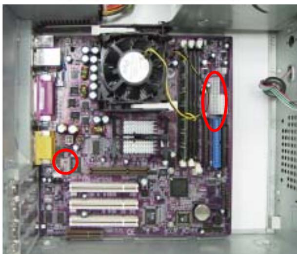
**3.** Locate the system board power connector. See figure for reference.
