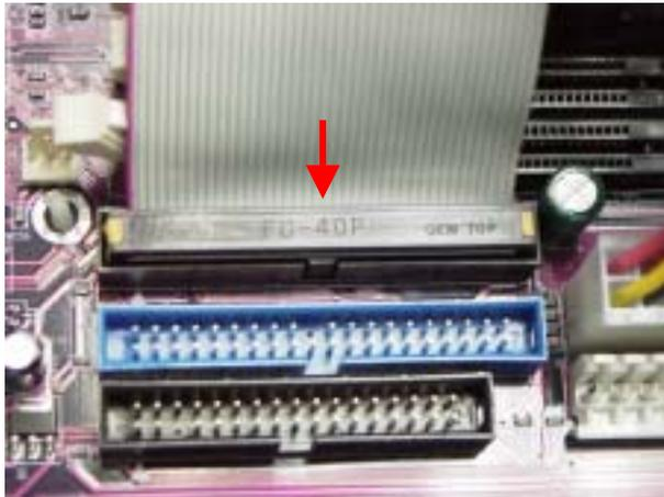
**9.** Plug the CD-ROM cable into the Primary IDE channel on the system board. The edge of the cable that is red determines its orientation. Push the CD-ROM cable squarely onto the Primary pins.
