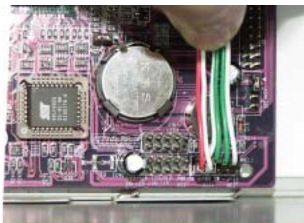
The Power SW and HDD LED should look like this after they are connected.
