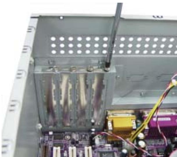
**1.** The most commonly used expansion card is the AGP and modem card. Let's start by installing the AGP card first. Remove the dust cover from the slot in the system case that corresponds to the expansion slot that you going to use.
