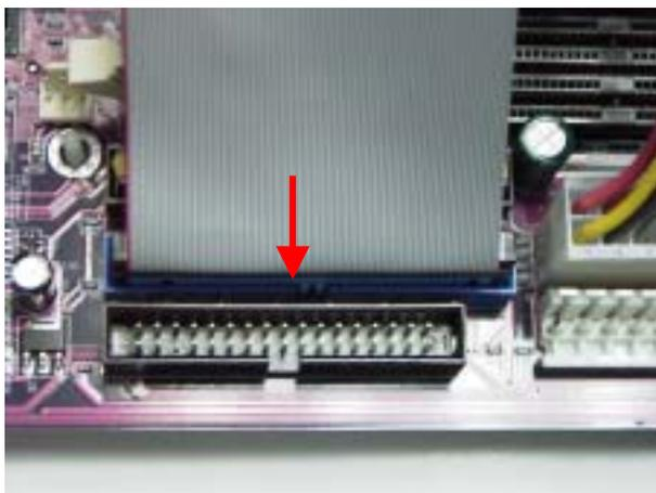
**11.** Next, plug the hard disk cable into the Secondary IDE channel on the system board. The edge of the cable that is red determines its orientation. Push the hard disk cable squarely onto the Secondary pins.
