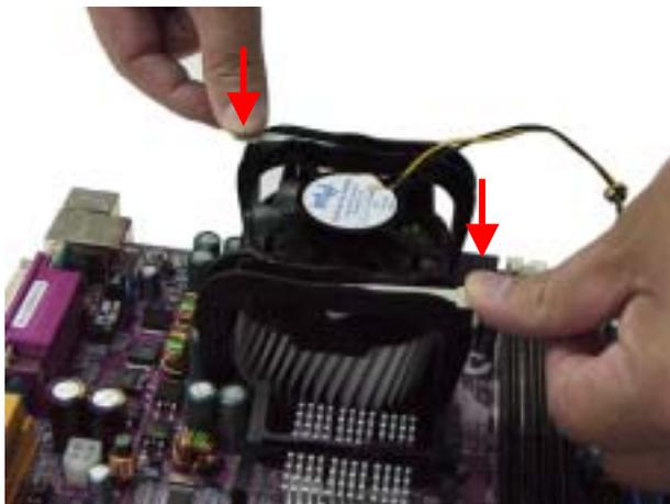
**7.** Lock both levers on top of the cooling fan to their opposite sides to secure the cooling fan on top of the heatsink.
