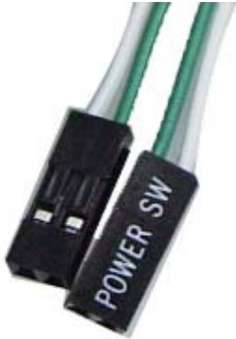
**1.** Connect the Power LED and Power SW cable on the Panel 1 of the system board. The Power button located in front of the case only works when the Power Switch connector is connected to the system board.
