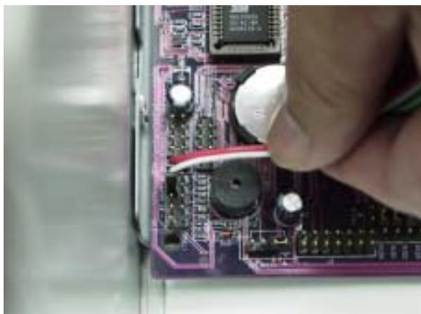
**4.** Next, Connect the HDD LED into the connector of the system board. The HDD LED indicator has two pins with one of them marked positive. One of the wires from the HDD LED is usually red and goes on the positive pin.
