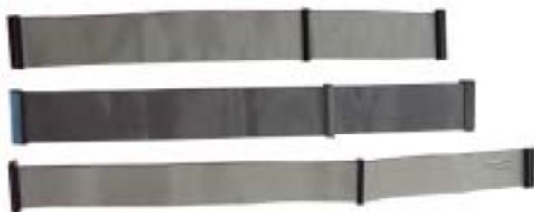
**8.** Next, you should get familiar with the cables that are used with the various drives. The first cable is use for the floppy drives, the second cable is for the hard disk drive and the third long cable is use for the CD-ROM drive.
