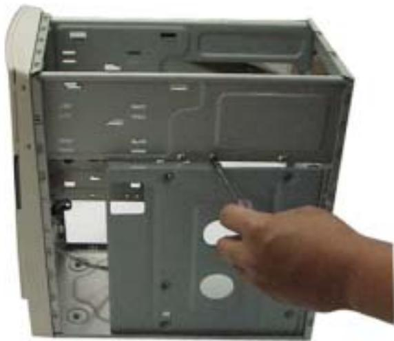
**4.** For installing the system board, locate the three screws which secure the plate and remove it.
