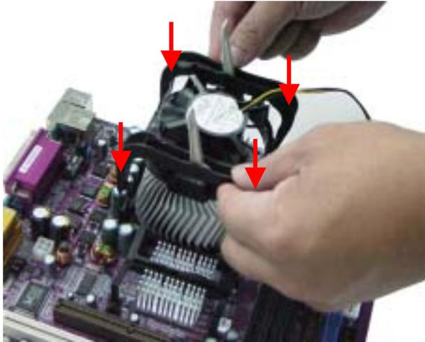
**6.** Attach the CPU cooling fan on top of the heatsink. Snap the four retention legs of the cooling fan into place.
