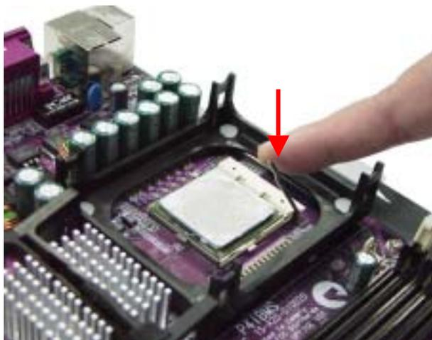
**4** Pull the CPU socket-locking lever away from the socket to unhook it and raise the locking lever to the upright position. Place the CPU into the socket and pull down the lever. Apply thermal grease to the top of the CPU.
