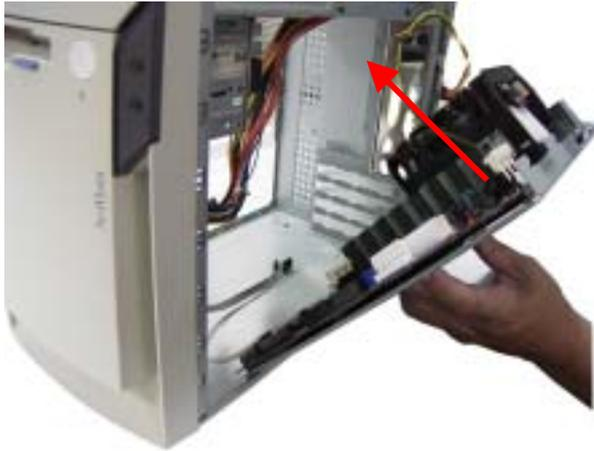
**12.**Place the system board over the mounting brackets. Then slide the system board into place as shown in the next figure.
