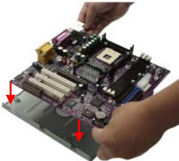
**2.** Position the system board in the plate so you can see the alignment of the mounting holes in the system board with the standoff holes. There are at least 4 screws that need to be secured.
