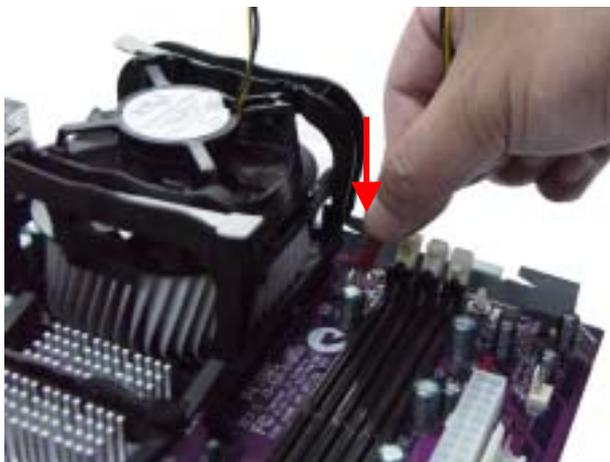
**8.** Connect the CPU cooling fan power cable to the CPU fan connector.
