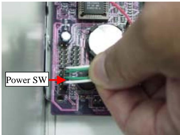
**2.** Connect the Power SW (usually with green wires) into the connector of the system board.
