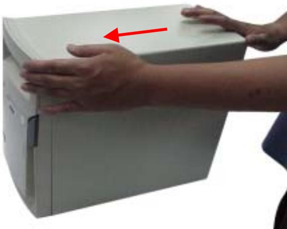
**2.** Using both hands, push the top cover towards the case. See figure for reference.
