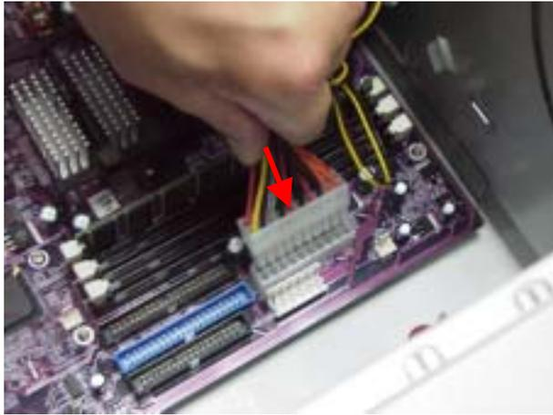
**4.** The power connector should fit perfectly in the slot on the system board. Note the orientation of the cables before trying to connect them. Each function of the cable is already defined.
