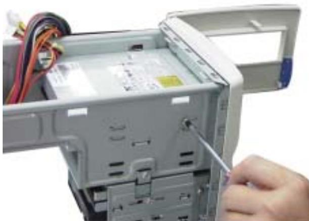
**6.** When the CD-ROM drive is positioned correctly, secure the drive to the bay using four screws.
