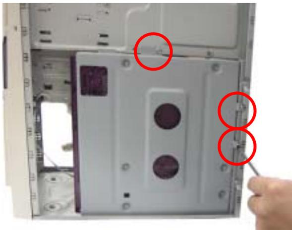
**13.**Secure the system board into the mounting brackets with screws. Do not overtighten the screws. Gentle pressure is enough.
