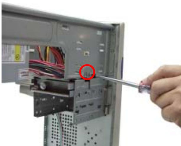
**1.** After you have installed the system board into the case, you should connect the power cable from the case power supply unit to the system board power connector. Since the floppy drive is situated closely to the power supply. For convenience purpose, loosen the screw that holds the Floppy drive.
