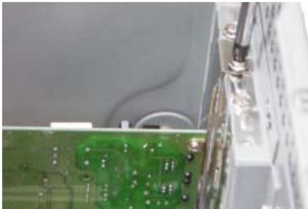
**7.** Secure the metal bracket of the Modem card with a screw.
