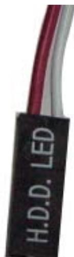
**3.** The HDD LED indicates the usage of the hard disk drives.
