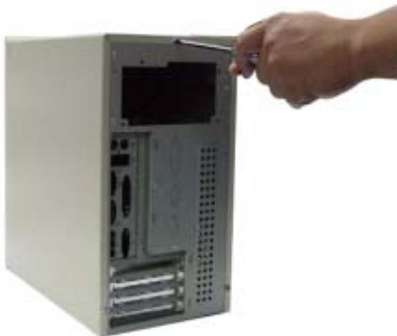
**2.** Locate the 3 screws at the back of the case; use the screwdriver to loosen them.
