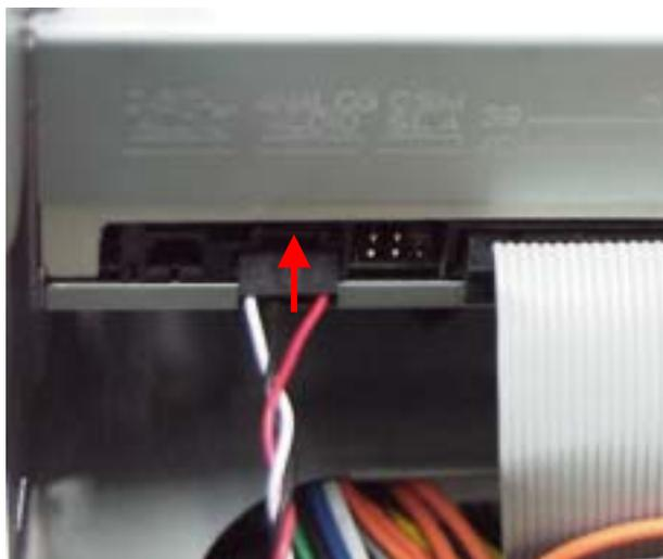
**15.** Use the audio cable provided with the CD-ROM drive to connect the audio connector on the rear edge of the CD-ROM drive to one of the audio-in connectors on the system board. The audio sound does not come from the system board itself.
