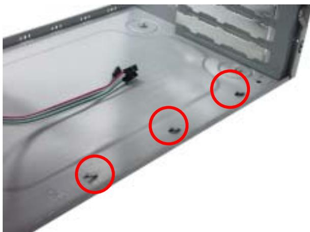
**11.**To install the system board inside the case. Locate the three mounting brackets on the case as shown in the figure.
