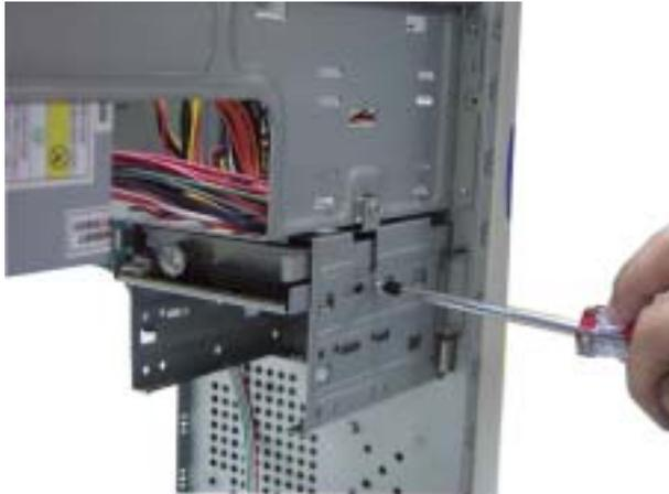
**2.** slide the drive in the appropriate location. For a 3.5" drive, secure the two screws located on the both side of the storage bay.
